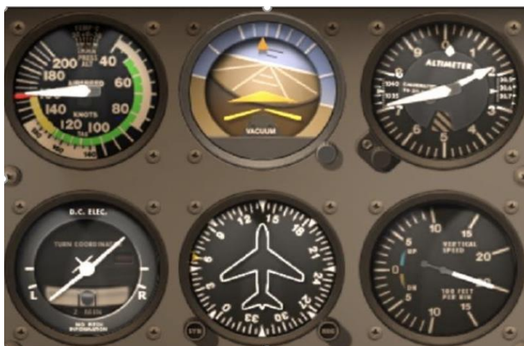
Figure 18: An example of the instrument panel of an aircraft in a spiral.
