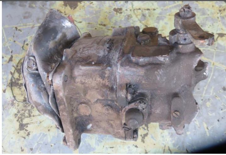
Impact damaged carburettor.
