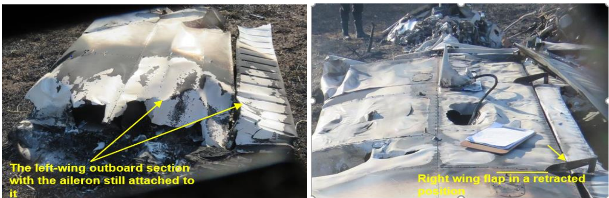
Figures 15/16: The left-wing outboard section (left) and the right-wing flap still in retracted position (right).
