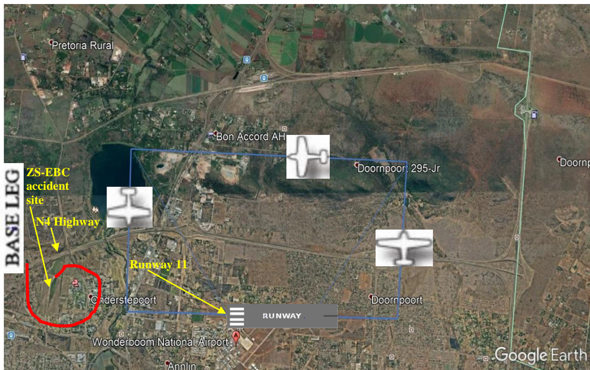
Figure 9: A map showing the standard training circuit pattern (blue colour) at FAWB, Runway 11. The red line shows the approximate flight path of ZS-EBC aircraft. (Source: Google Earth)
