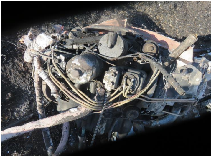
The engine, a Lycoming O-360-A30 engine, Serial No. L-6678-36.
