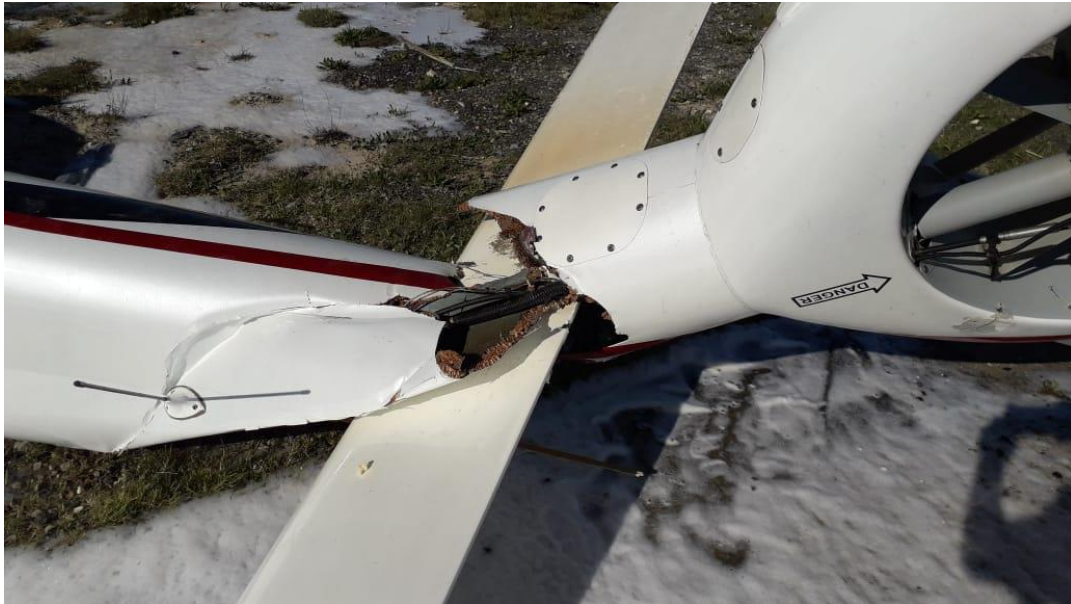
Figure 4: The broken tail boom structure on the front part of the fenestron. (Photograph courtesy of FACT ARFF)
