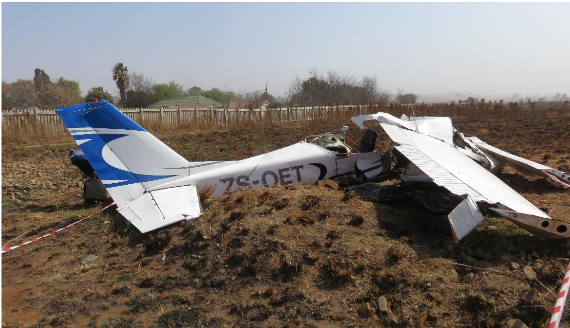
Figure 3: The aircraft as it came to rest in an upright position on its belly.
