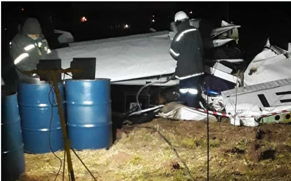
Figure 14: Spill response company members draining fuel from the right-wing tank into a 210L drum.
