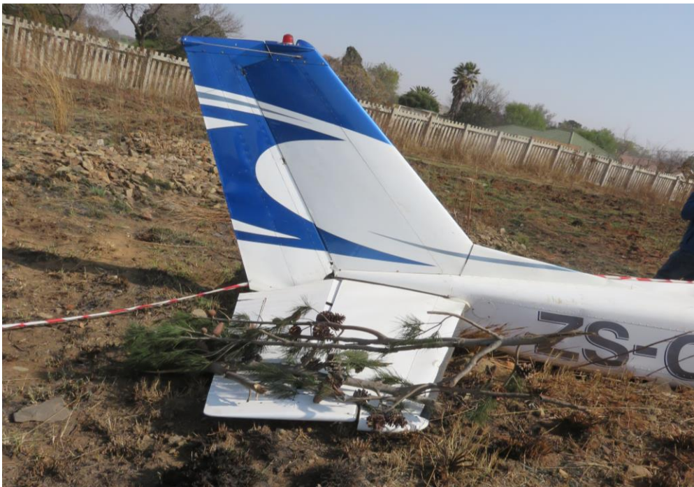
Figure 11: Tree branches on the horizontal stabiliser from the tree with which the aircraft collided.
