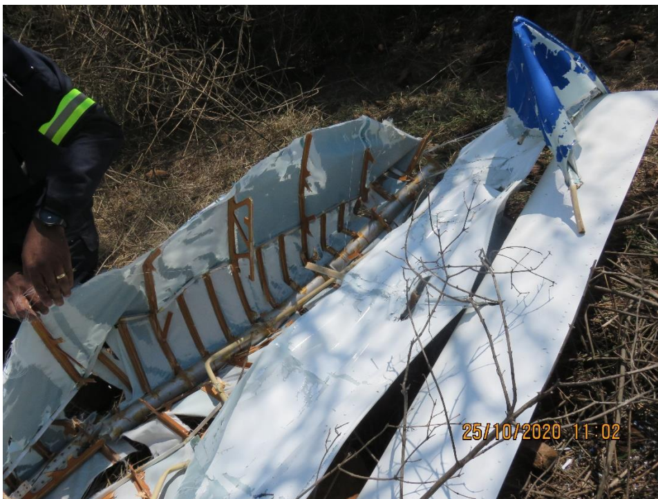
Figure 9: The damaged main left-wing spar.
