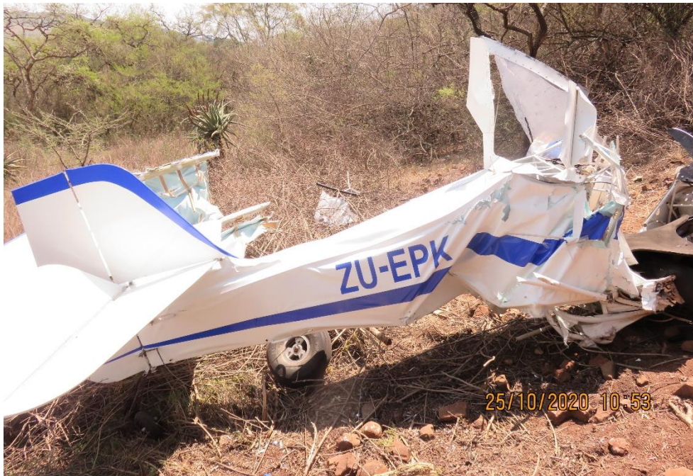
Figure 10: Wrinkles on the fuselage due to impact forces.
