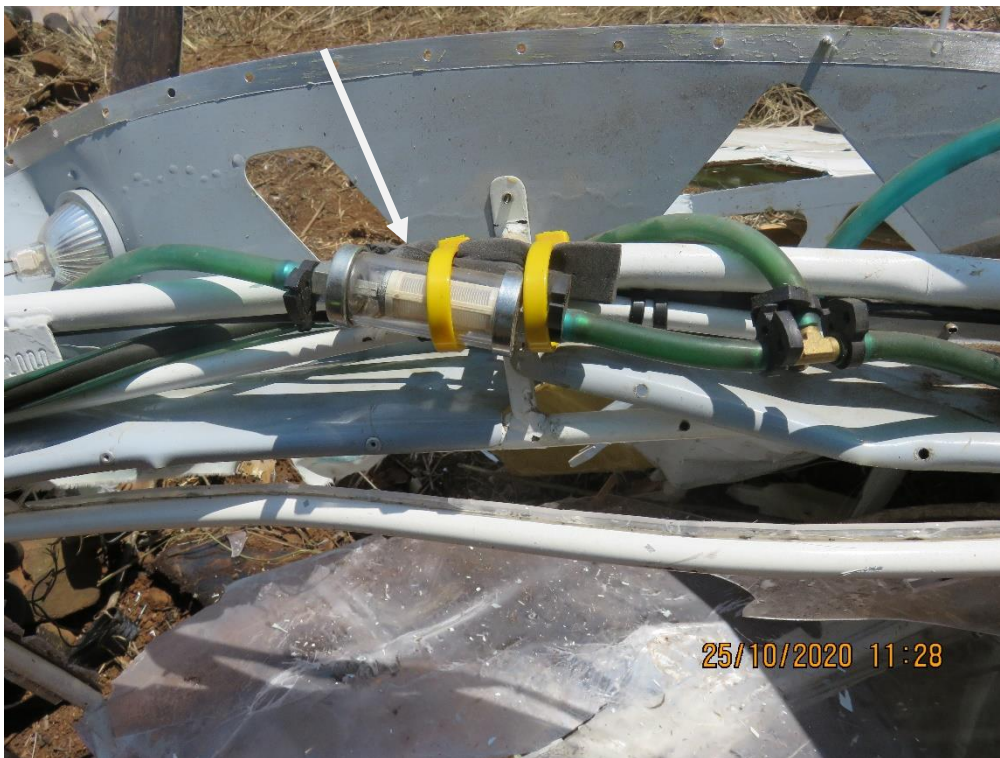
Figure 12: Arrow showing an empty or dry airframe fuel filter.
