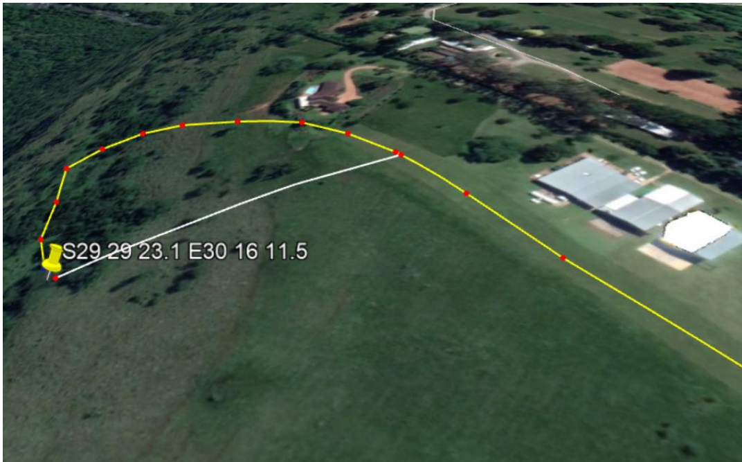
Figure 7: The airstrip elevation is 3453ft and the accident site elevation is 3356ft. The white line shows a distance of 130.83m from the crash site to the runway threshold.
