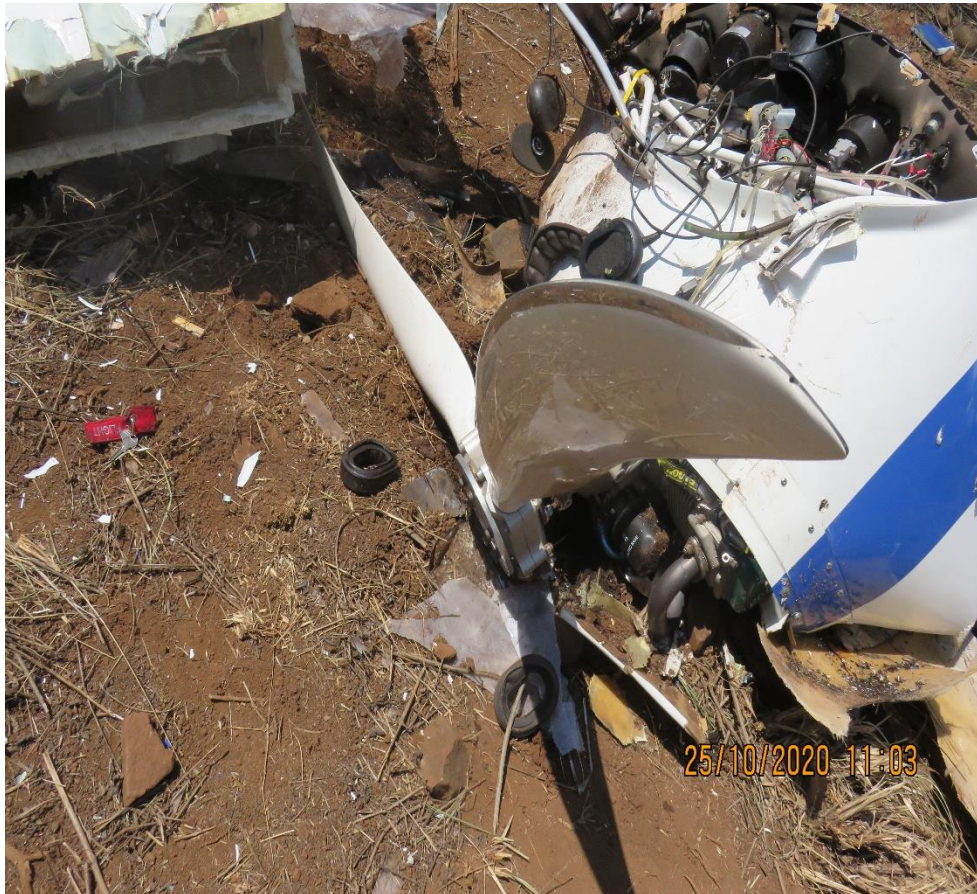
Figure 11: Two of the three propeller blades were still intact.
