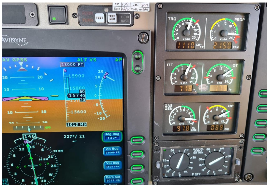
Figure 1: The engine instruments indicating normal operation during the climb.
