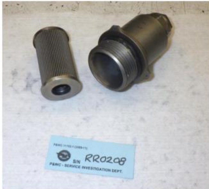
Figure 9: The fuel filter after it was removed from the filter housing.
