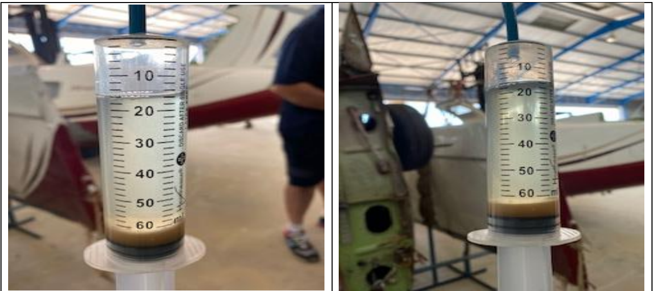
Figure 7: Contaminated fuel drained from the right-wing collector tank.
