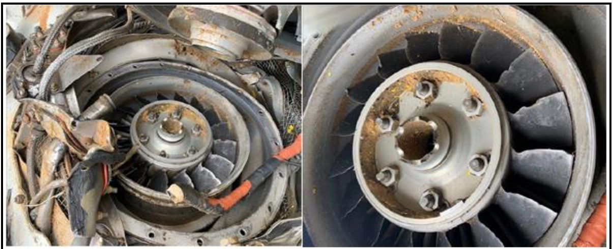
Figure (13&14): Shows the damages on the compressor rotor blades
