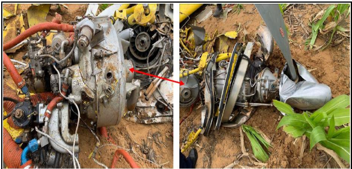
Figure s9 and 10: Engine inlet stuts, liberating the accessory gearbox.
