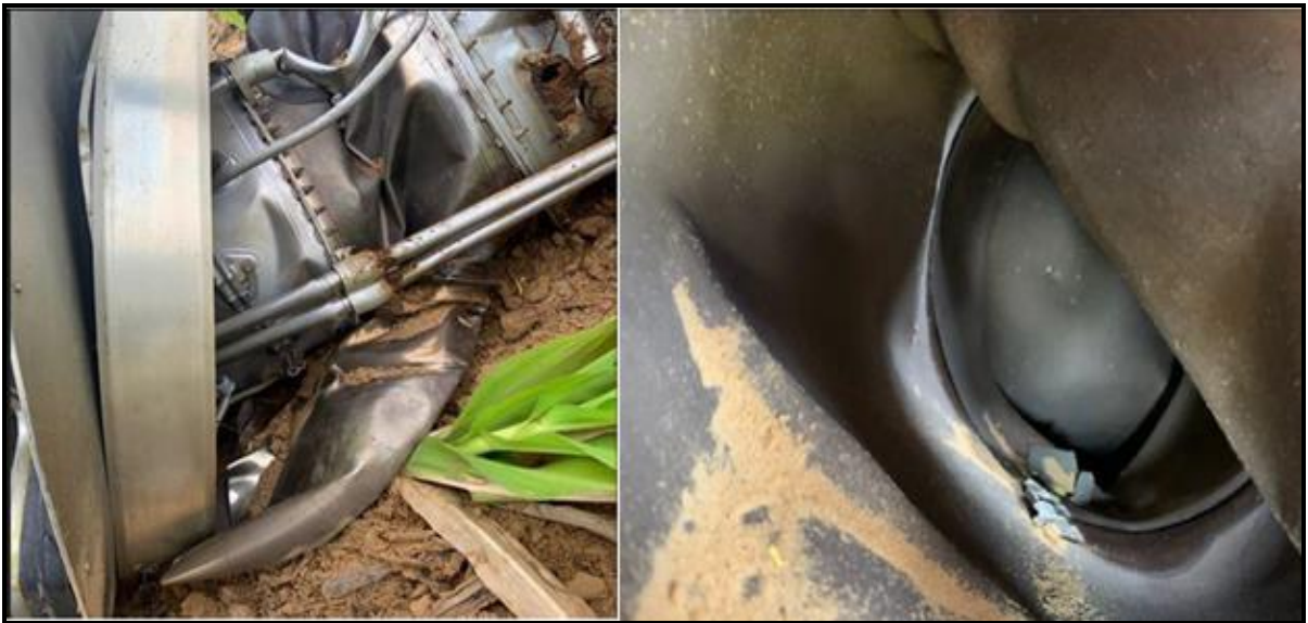
Figures (11 and 12): Damage of the exhaust case (left); PT blades fragment in the exhaust case (right)
