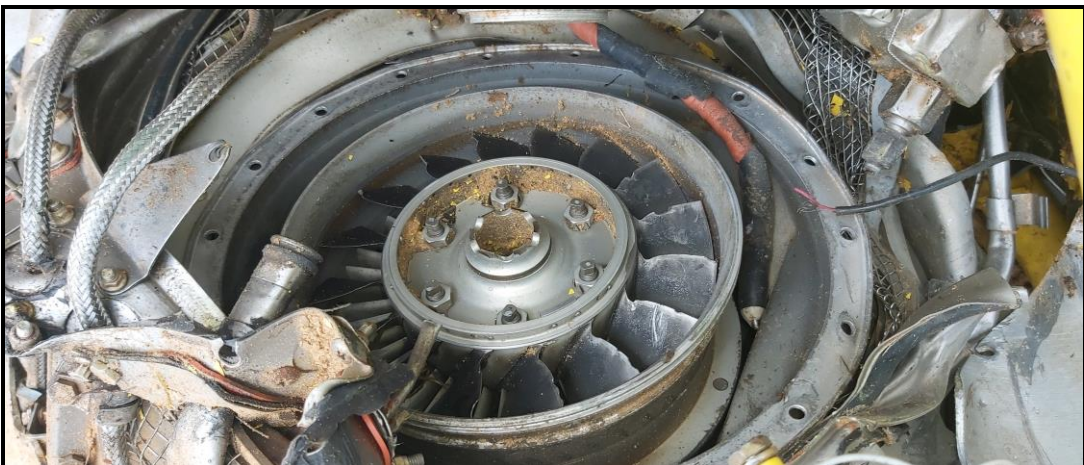
Figure 7: Damage on the engine turbine blades section.
