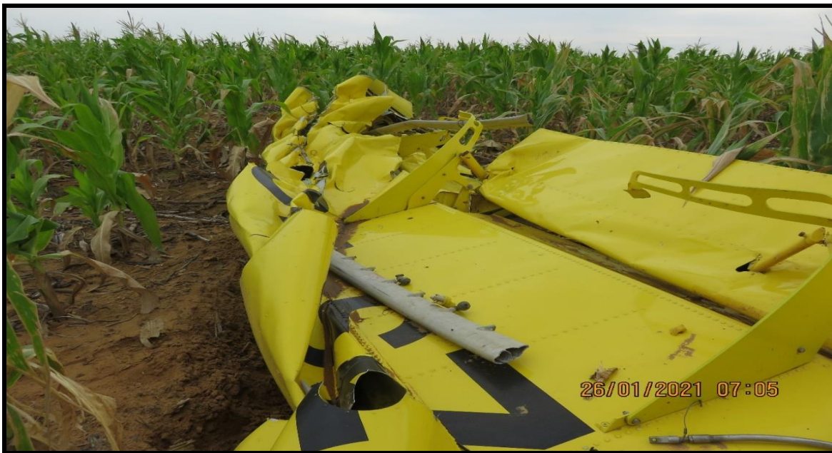
Figure 4: The damaged left wing due to impact.
