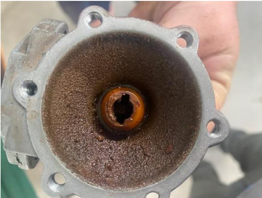
Figure 3: Mechanical fuel pump with sludge.
