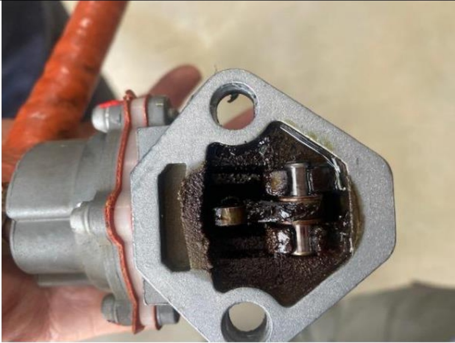
Figure 2: Visible sludge inside the mechanical fuel pump.
