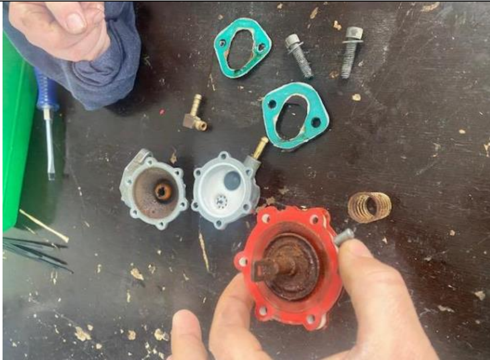
Figure 4: Sludge in the mechanical fuel pump.
