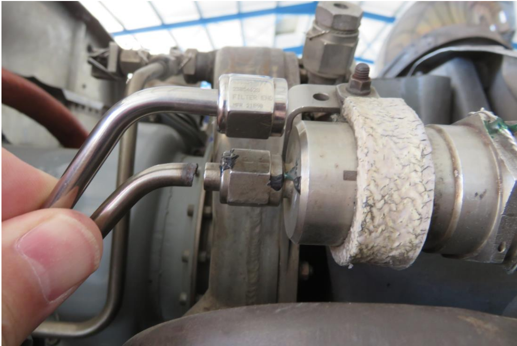
Figure 10: Comparison between the long end (new tube, top) and the short end (failed tube).
