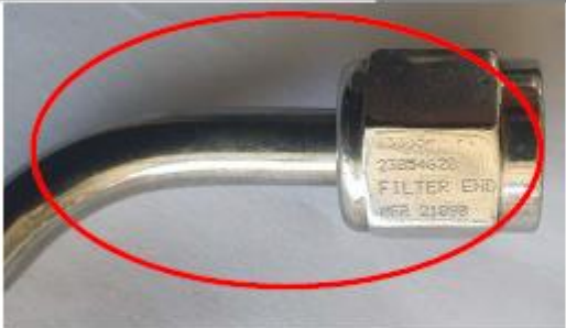
Photo 8: Reference Tube showing a variation of "Filter End" inscription (Digital)
