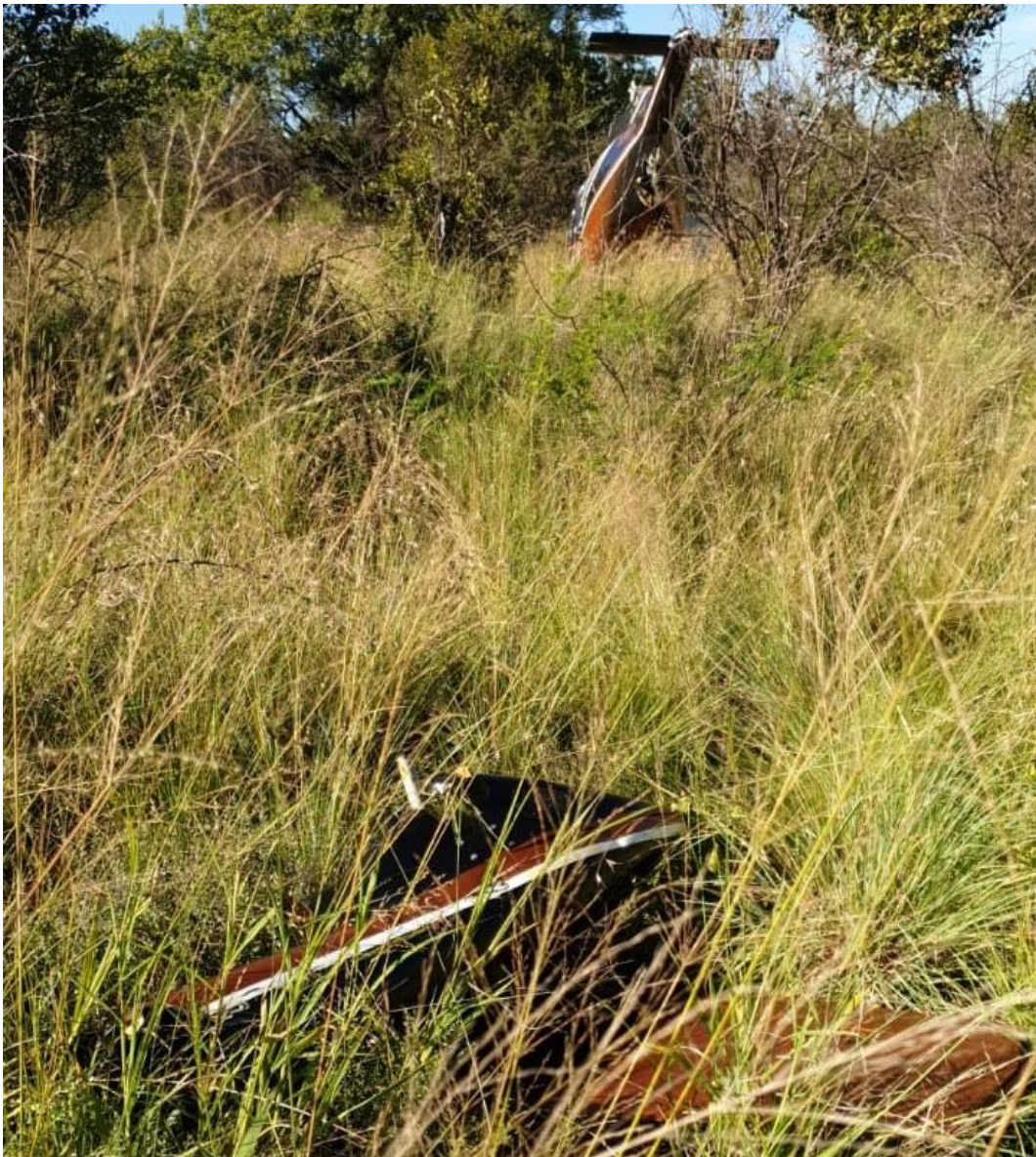
Figure 4: An aft view of the helicopter as it came to rest with the aft tail boom in the foreground.
