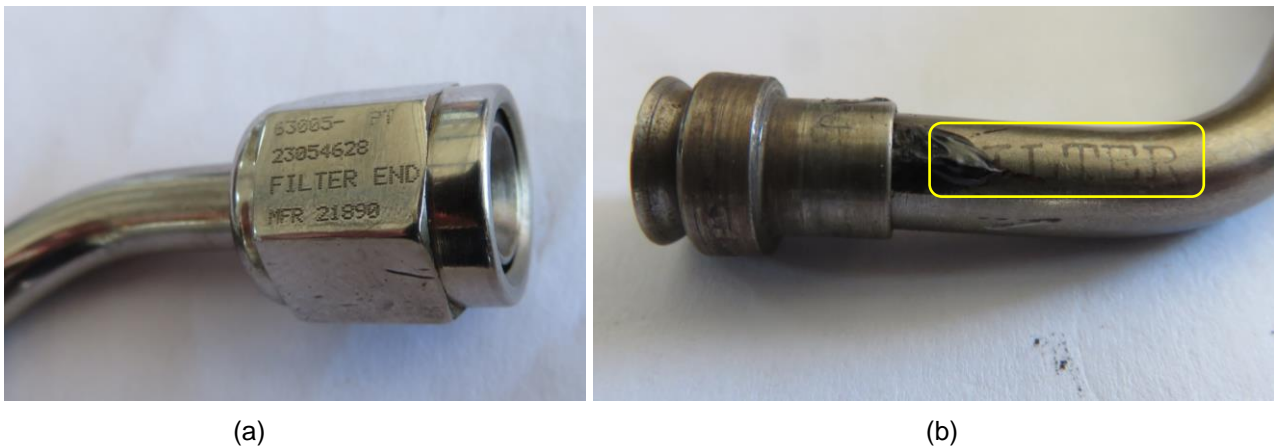
Figure 9: (a) The new Pc tube: (b) The Pc tube removed from the accident helicopter engine.
