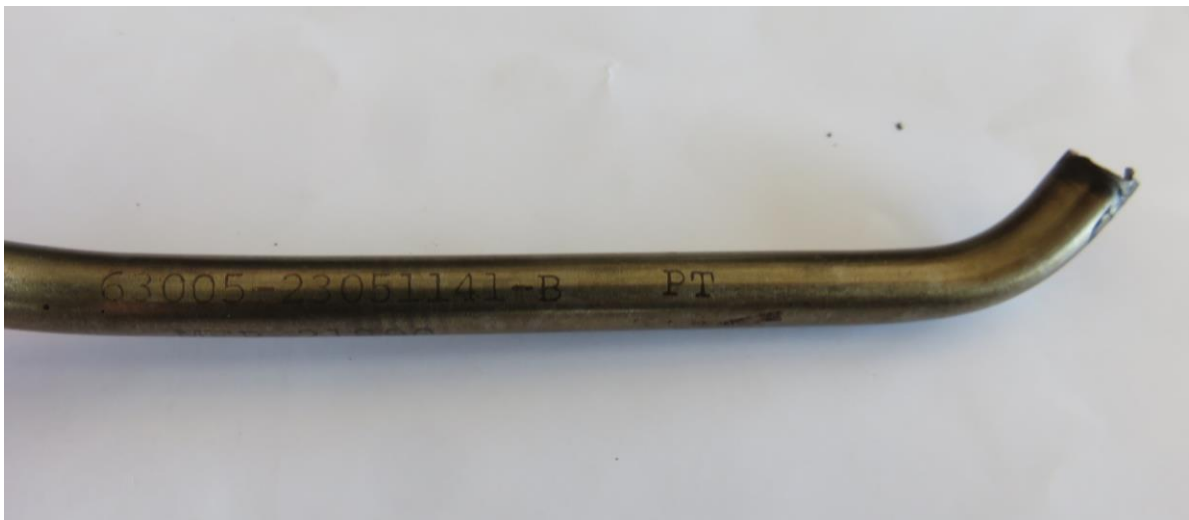
Figure 6: The fractured Pc tube with part number 63005-23051141-B printed on it.
