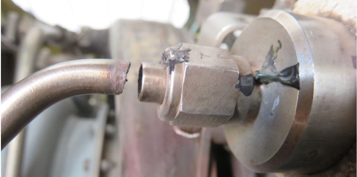
Figure 7: The fractured Pc tube (forward connection of the Pc filter) as it was found on the engine.
