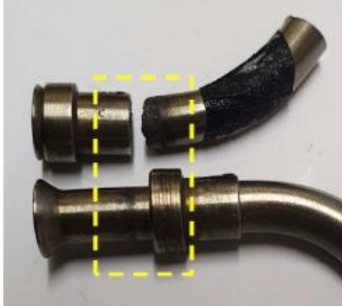
Photo 5: Tube opposing ends showing corrosion damages (Digital)
