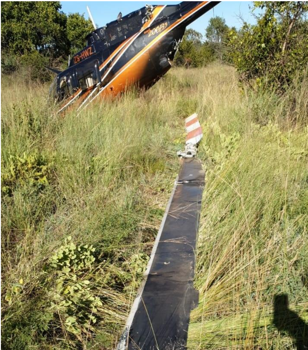
Figure 5: The entire main rotor assembly had separated from the main rotor drive shaft.
