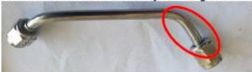
Photo 7: Reference assembly showing correct fitment orientation (Digital)
