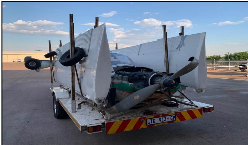
Figure 3: Damaged propeller blades.
