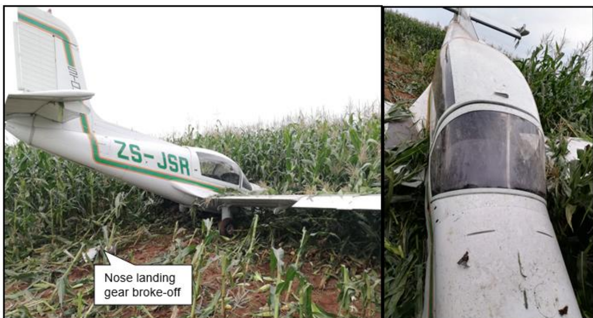
Figure 2: The damaged aircraft as it was found at the accident site. (Source: Picture courtesy of the pilot)
