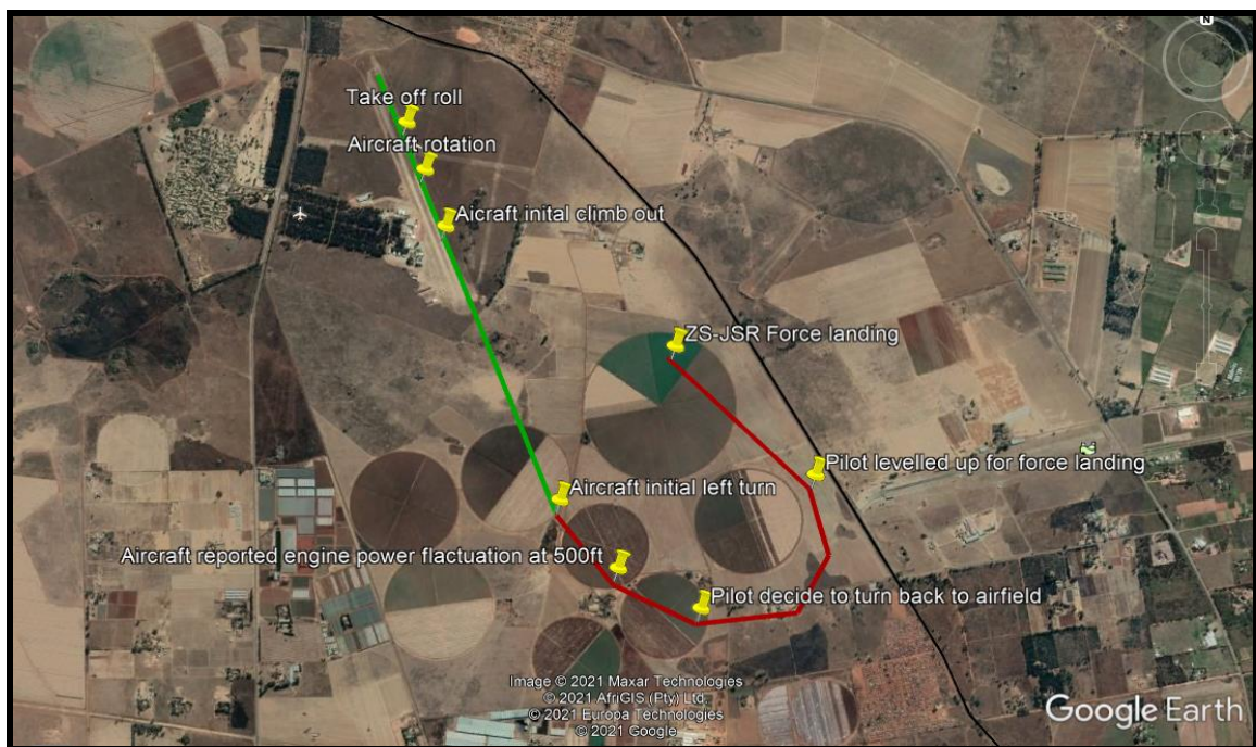
Figure 1: The aircraft's route from take-off to turn back point. (Source: Google Maps)
