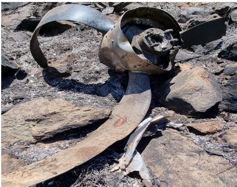
Figure 9: Fractured driveshaft and the propeller showing curled blades.
