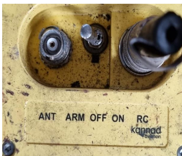
Figures 13/14: The Kannad 406 ELT and the position of the switches.
