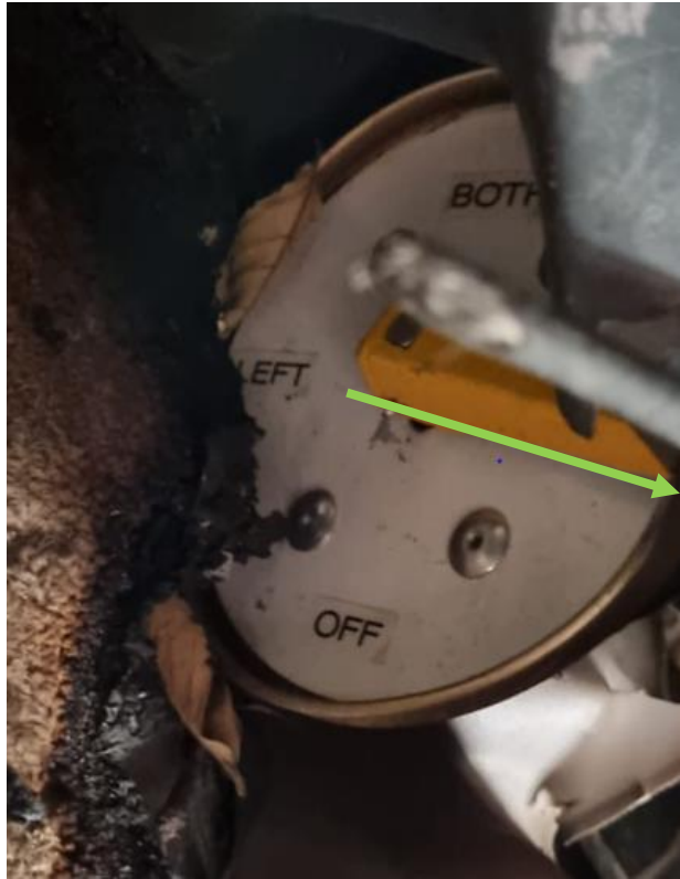
Figure 8: The fuel selector set to the right tank.
