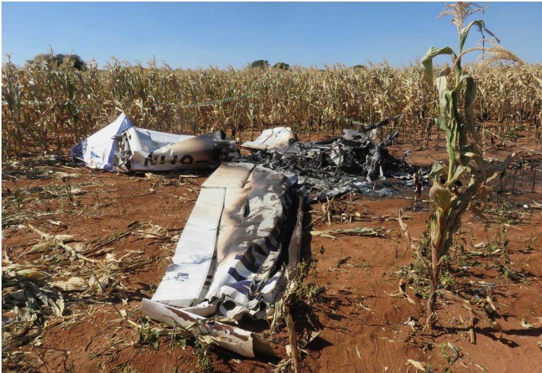
Figure 3: The wreckage of the ZS-OMN aircraft as it came to rest in an inverted attitude.
