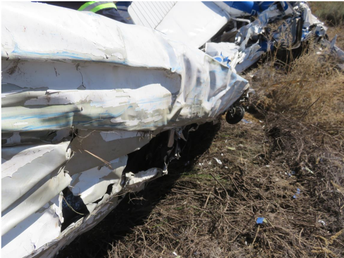
Figure 17: The compressed left-wing leading edge of the ZS-PXI that impacted the ZS-OMN, leaving traces of the blue paint of the registration mark on it.
