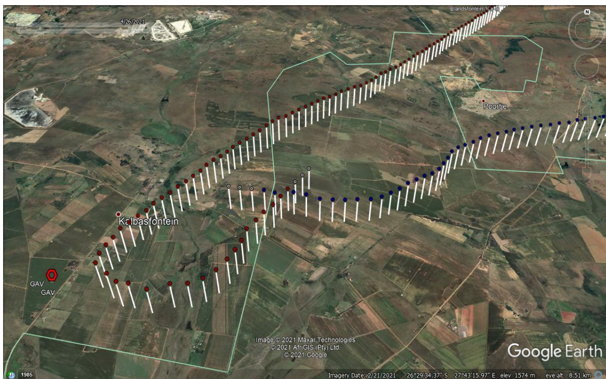
Figure 1: Radar data showing the ZS-PXI path in red dotted track; and ZS-OMN path in blue dotted track. (Source: ATNS)
