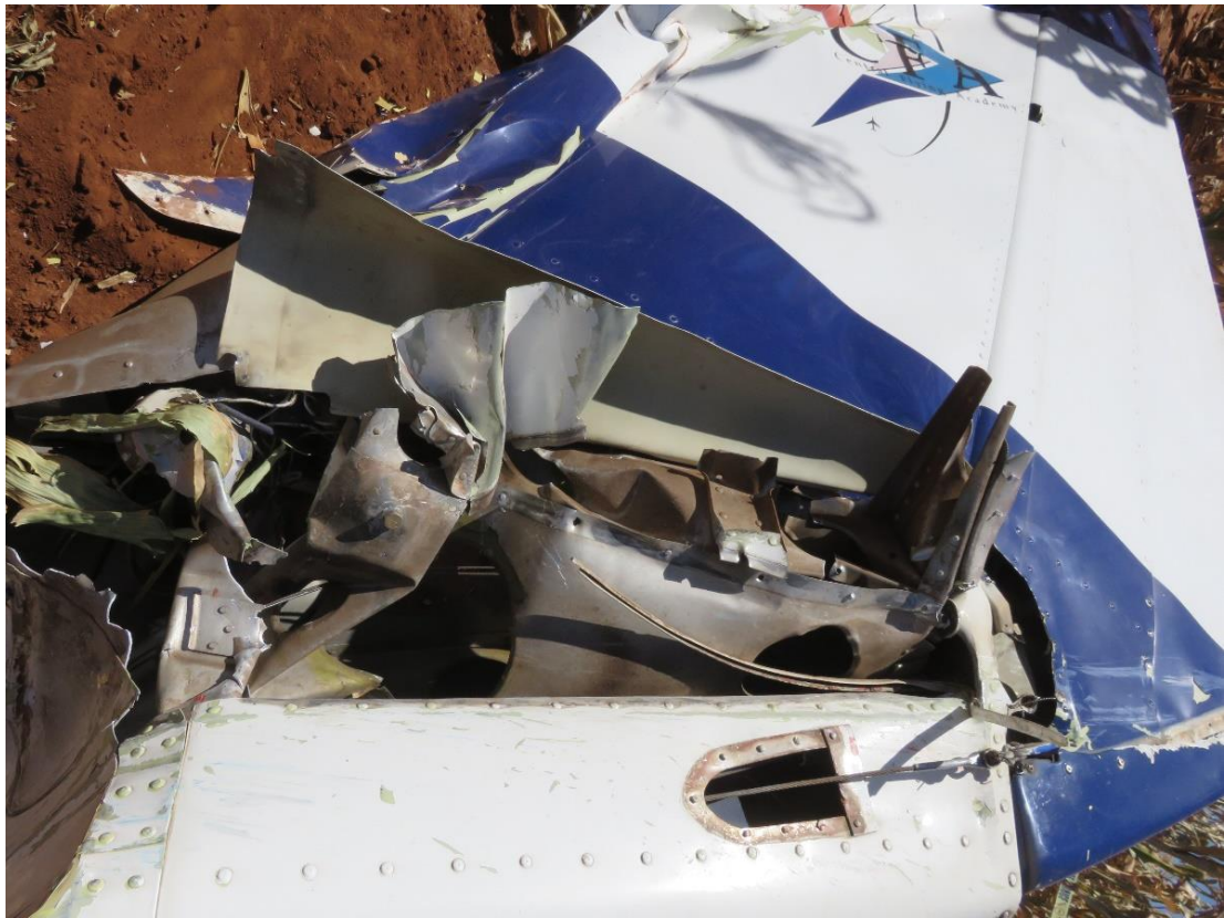
Figure 11: The empennage of the ZS-OMN displaying the hardware deformation where the left horizontal stabiliser was installed.
