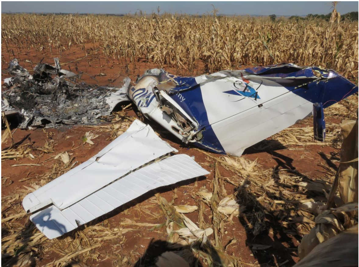
Figure 18: The left horizontal stabiliser was recovered and placed in position during reconstruction.
