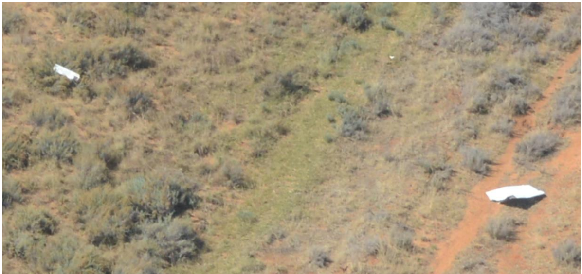
Figure 12: The left ZS-PXI left-wing tip fairing on the left of the picture, and the ZS-OMN horizontal stabiliser on the right of the picture.
