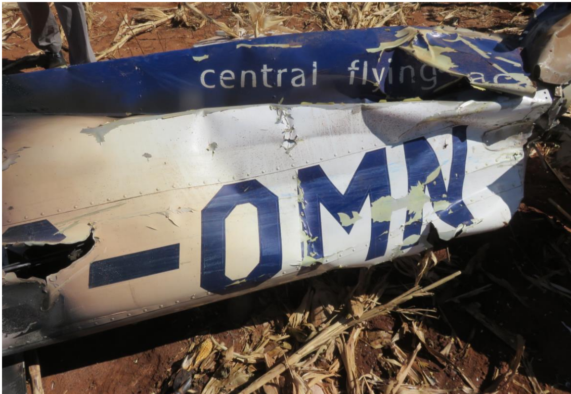
Figure 16: The impact markings caused by the left-wing leading edge of the ZS-PXI on the left aft fuselage of the ZS-OMN.
