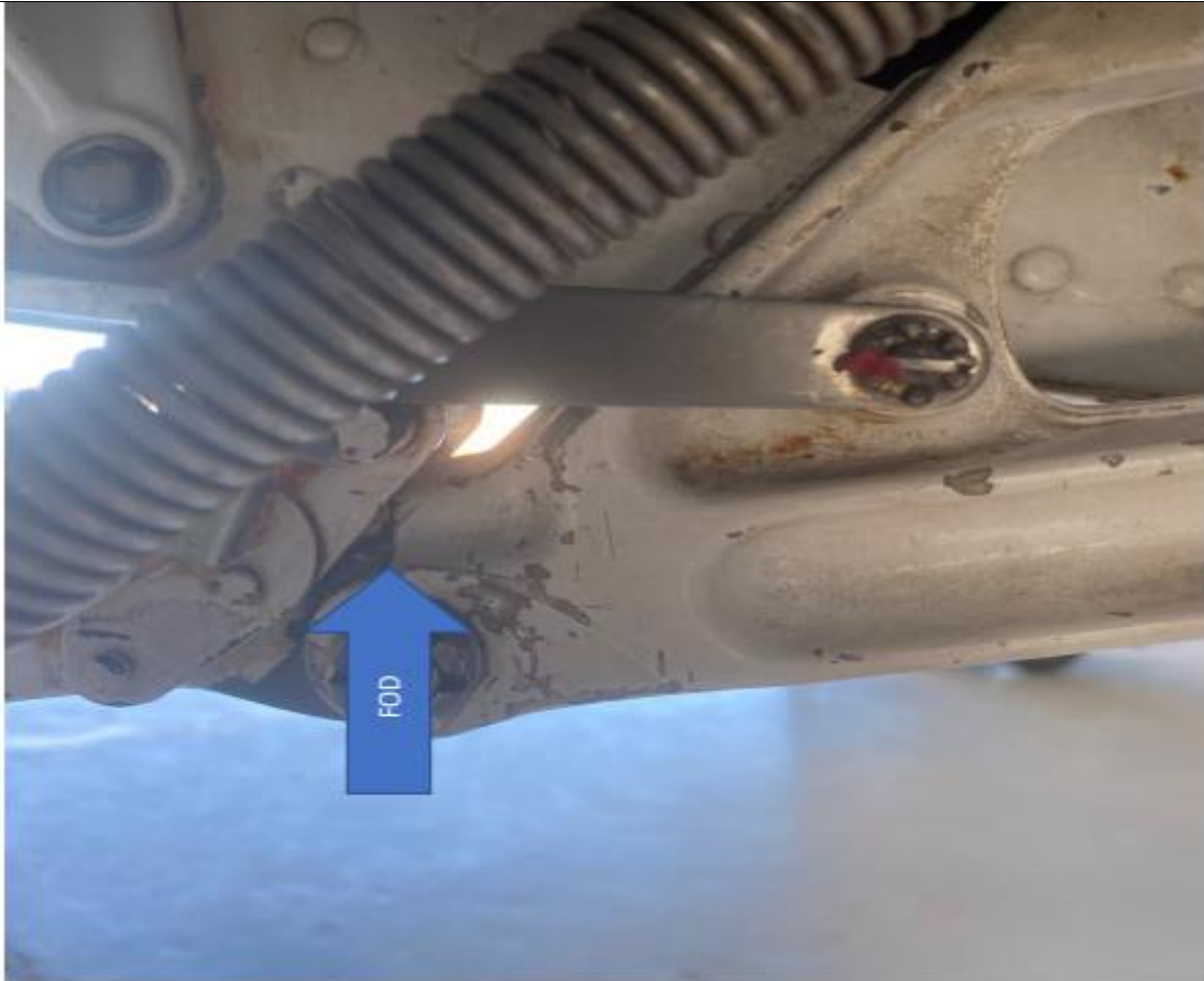
Figure 3: An arrow indicates where the FOD was stuck on the left-side main gear.
