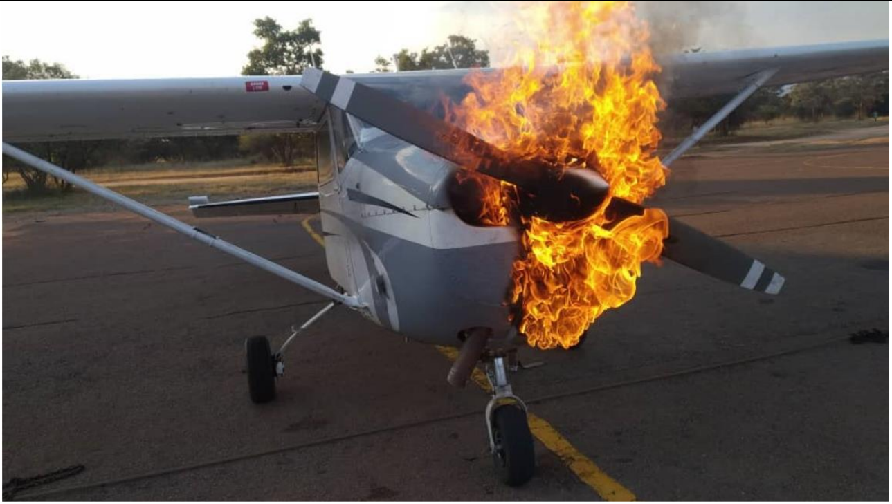
Figure 1: Front section of the nose compartment that caught fire. (Source: Pilot)
