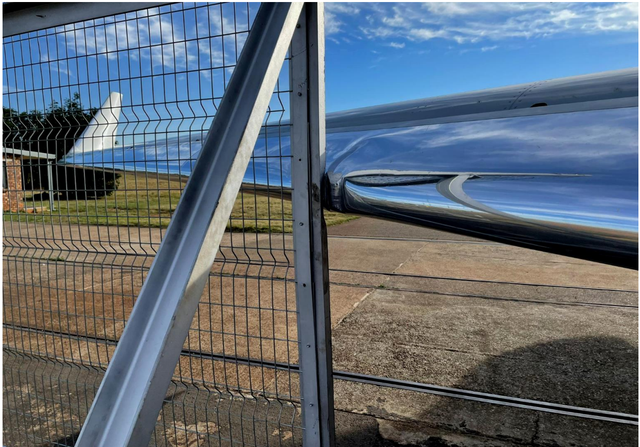
Figure 9: The gate whilst in contact with the leading-edge slat. (Source: Fireblade Aviation)
