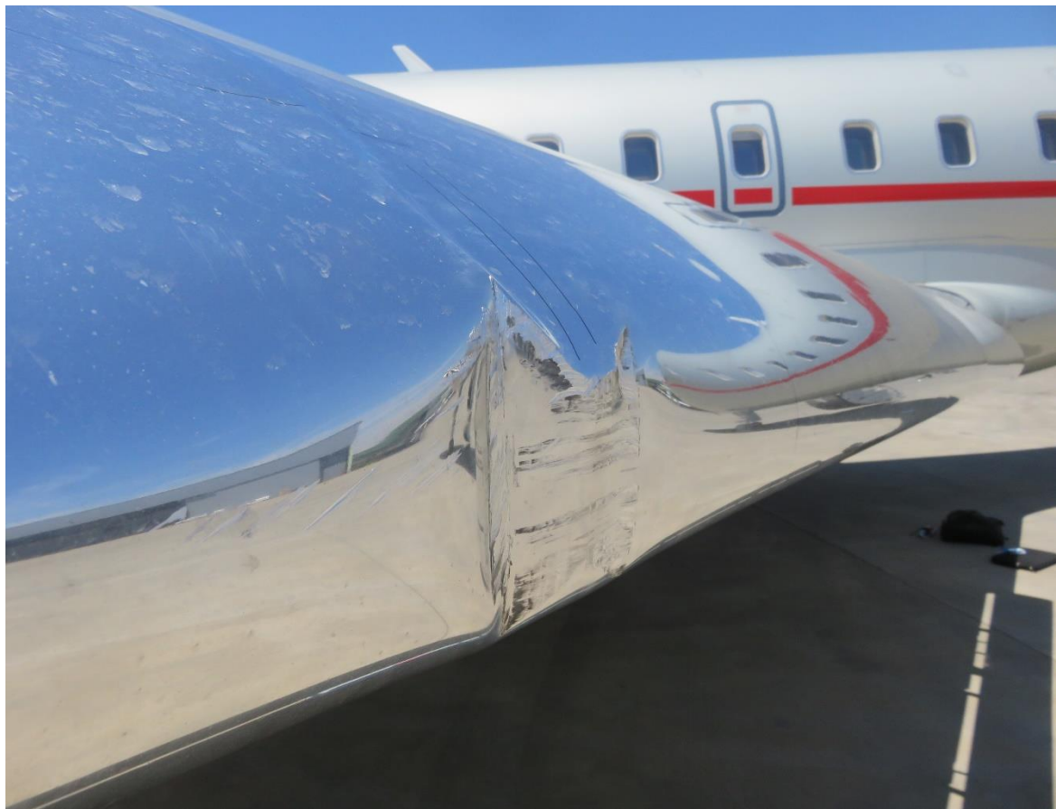
Figure 3: Deformation of the number 2 leading edge slat on the right wing.
