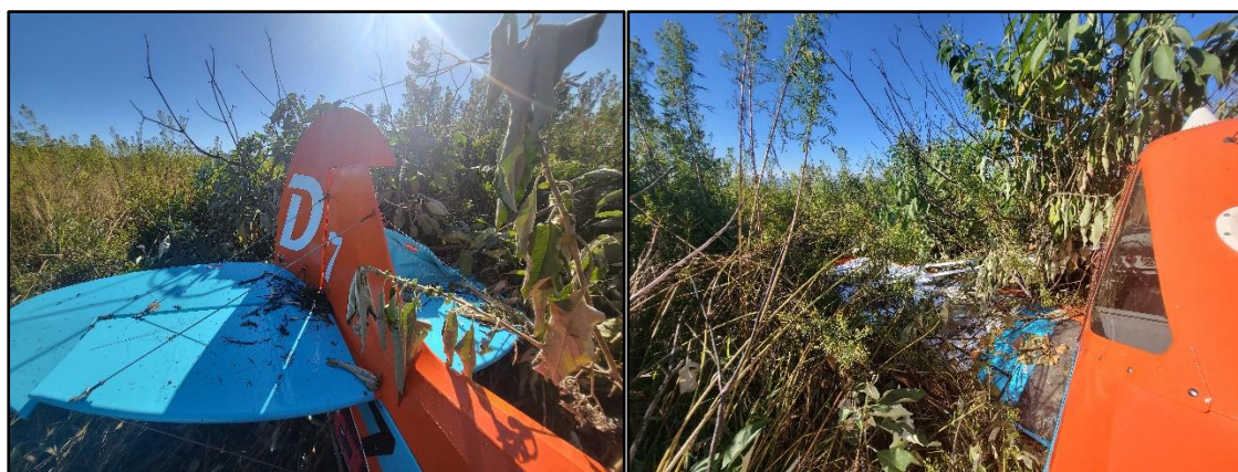
Figure 6 and 7: Damage to the left elevator (left); and left-side wing embedded in the bushes (right).
