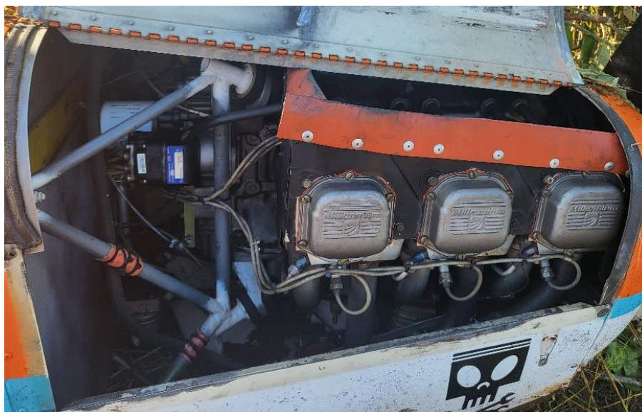
Figure 8: The condition of the engine compartment as it was found at the accident site.
