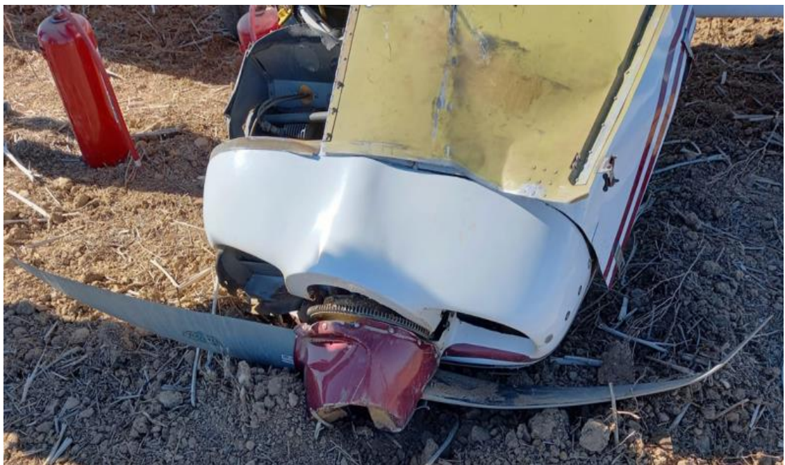
Figure 5: The damaged propeller hub and propeller blades.
