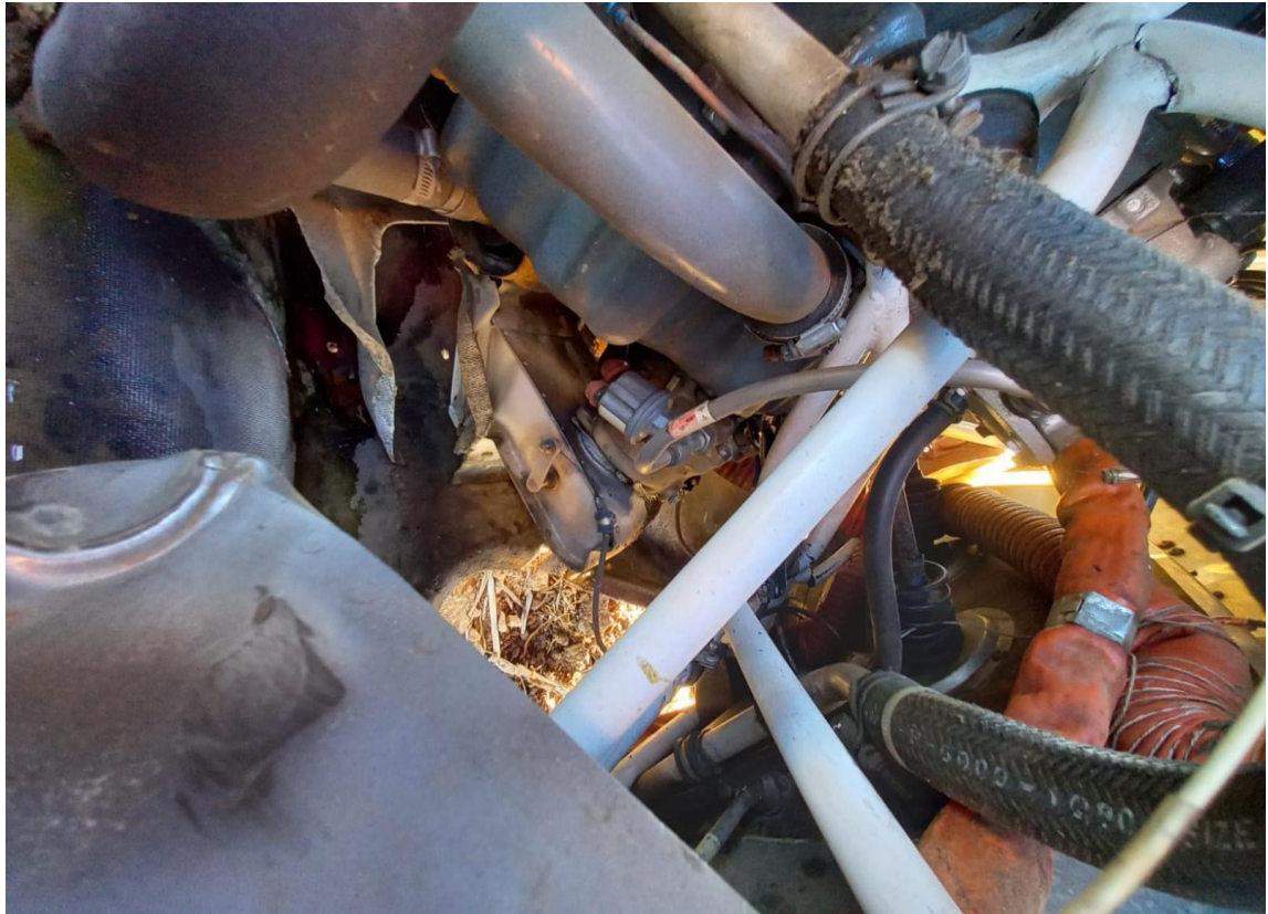
Figure 6: Damages sustained in the engine compartment and bent engine mountings.
