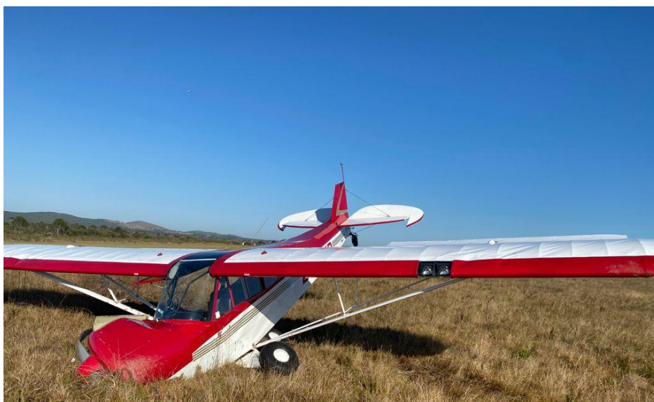
Figure 3: The aircraft sustained damage to the propeller, landing gear and fuselage.
