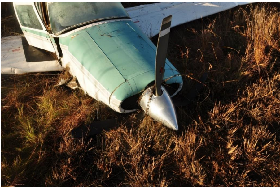
Figure 8: The propeller with the barbed wire fence around it. The propeller blades indicate that the engine was not under power during impact.
