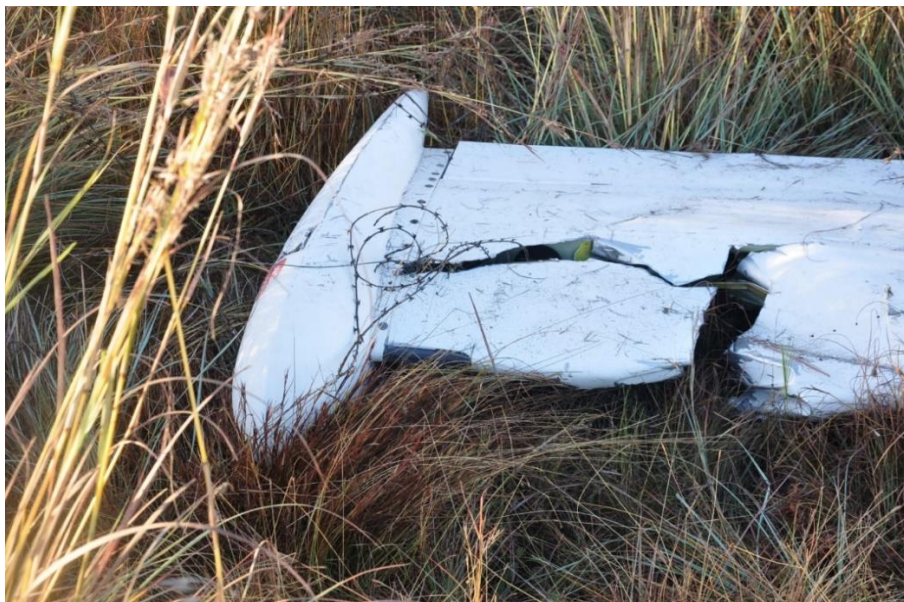
Figure 7: The right wing that hit the fence post.
