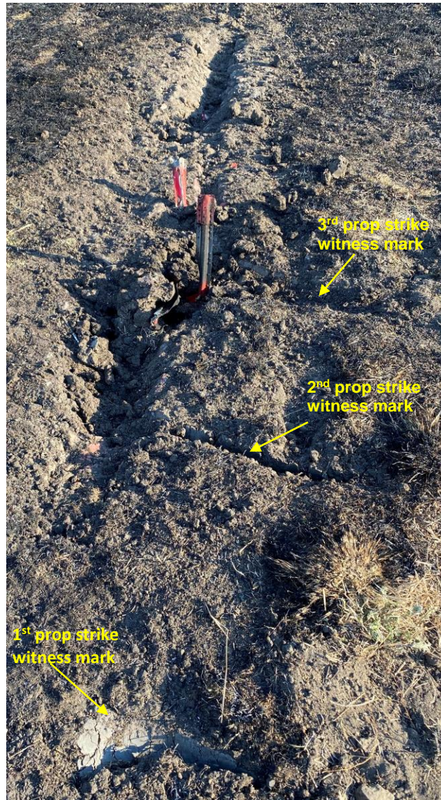
Figure 11: Ground marks left by the aircraft's blades.
