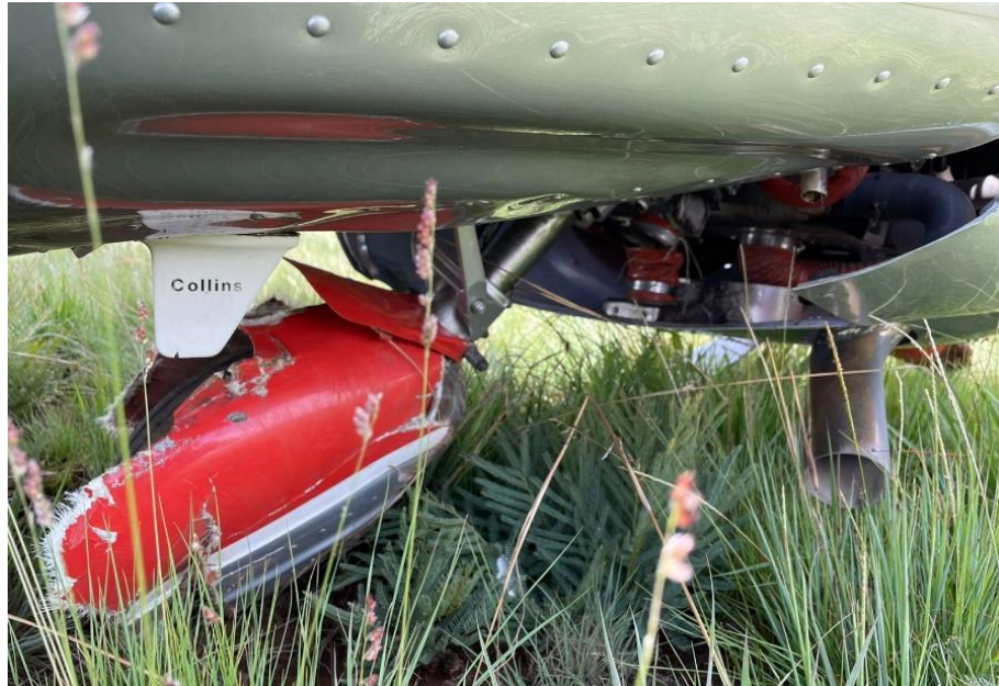
Figure 5: Damaged nose landing gear strut. (Source: Pilot)
