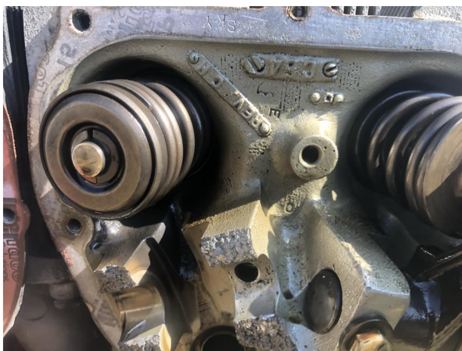
Figure 4: Damaged caused to the number 5 cylinder boss.
