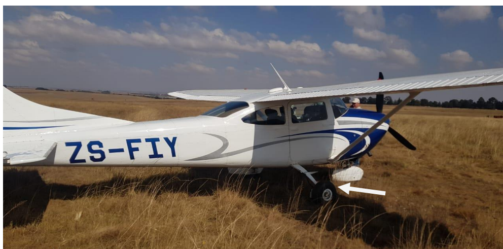
Figure 3: Damaged wheel fairing post-incident.
