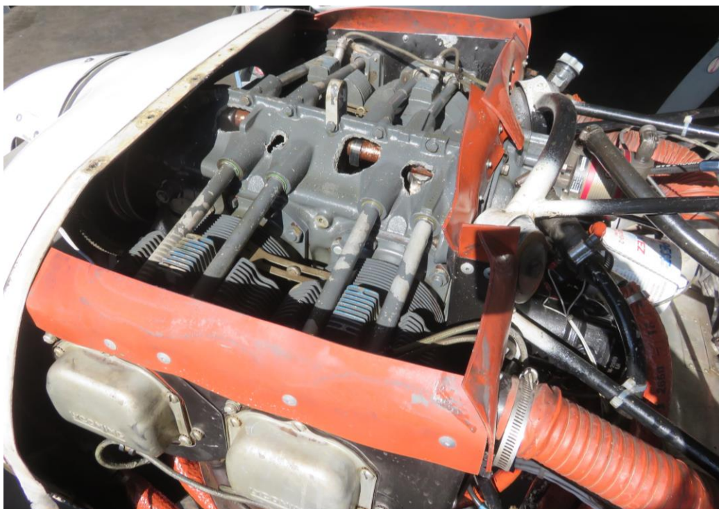
Figure 3: Damage to the engine crankcase.
