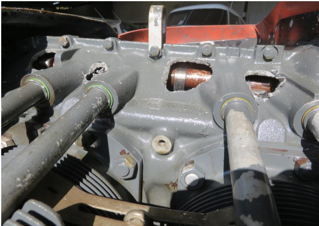
Figure 7: A closer view of the damaged crankcase.
