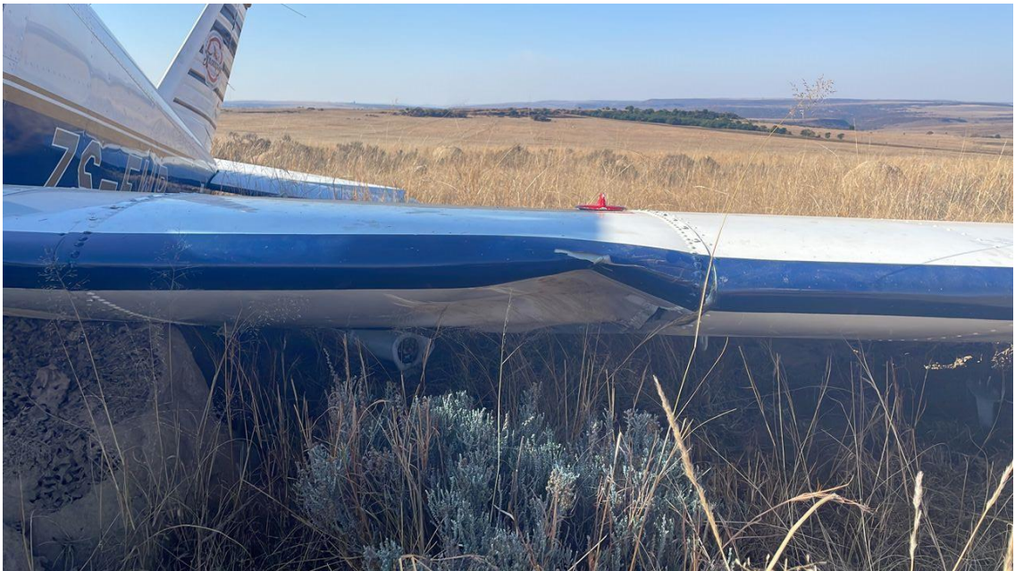
Figure 5: Damage to the left wing caused by the main gear strut that broke off. (Source: Pilot)
