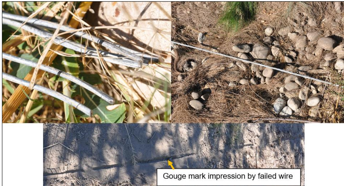
Figure 17: Top-left image: The failed earth conductor. Top-right image: The earth conductor found near the trees. Bottom image: The gouge mark made by the earth conductor after failure.
