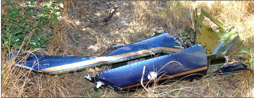
Figure 12: Tail boom middle section (original position).
