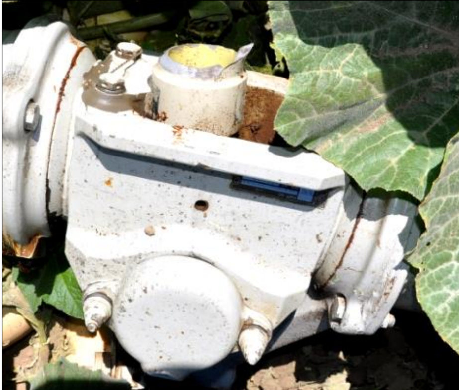
Figure 10: Damage to the main rotor mast.
