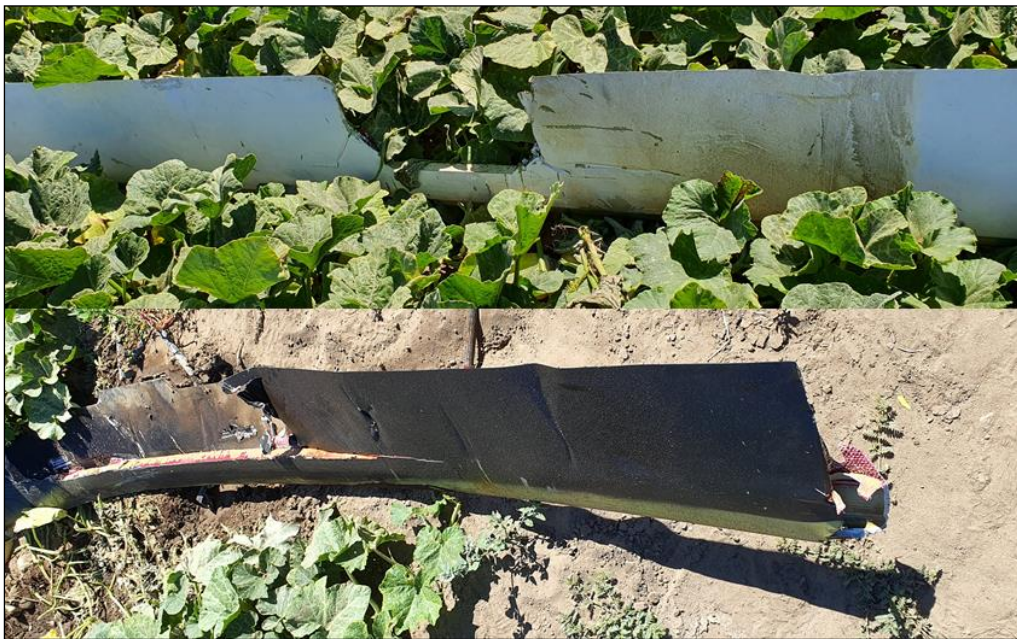
Figure 9: Damage to the main rotor blades.
