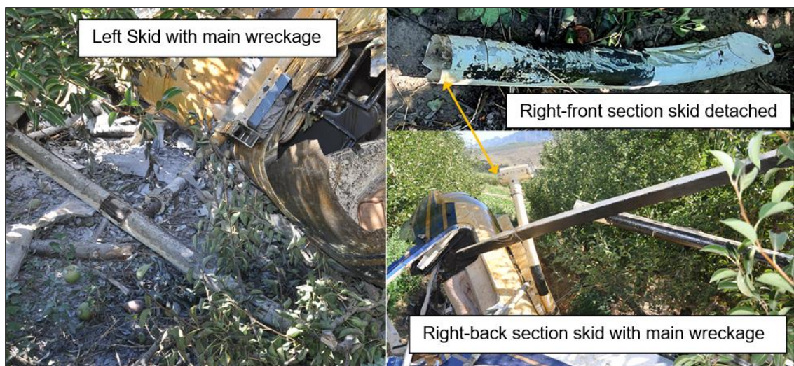
Figure 16: Left image: The left skid still attached to the main wreckage. Top-right image: The front section of the right skid showing striations marks. Bottom-right image: The right skid after the accident.
