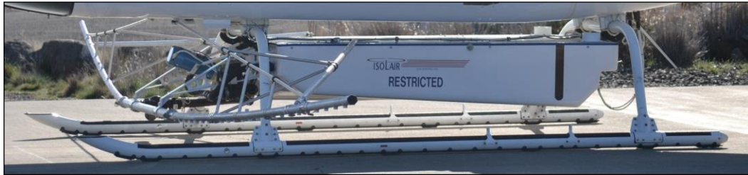
Figure 6: An IsoLair system installed on a similar helicopter as the accident helicopter. (Source: http://www.isolairinc.com/index.php )
