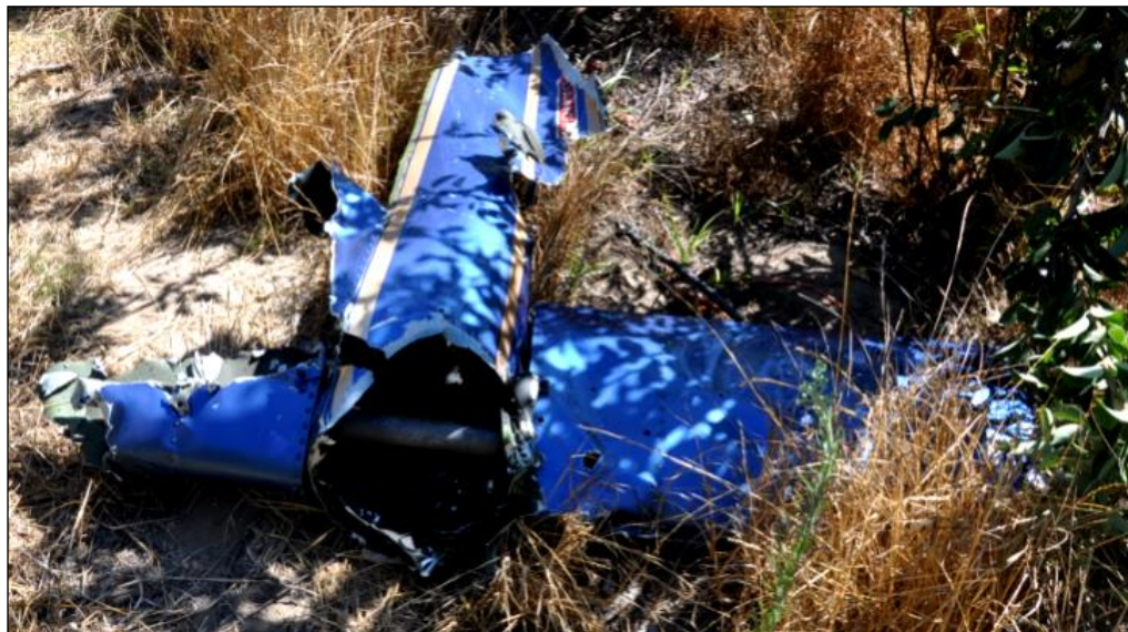
Figure 13: Horizontal stabiliser section (original position).
