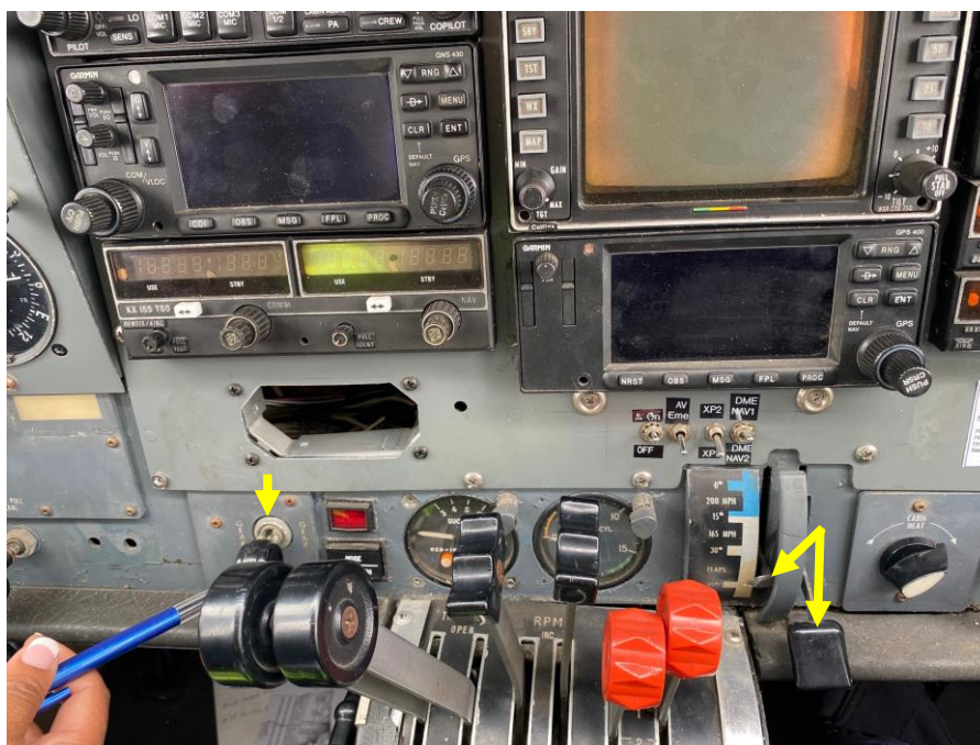
Figure 9: View of the aircraft console showing the landing gear lever selected in an extended position and the flap lever at 45° setting.
