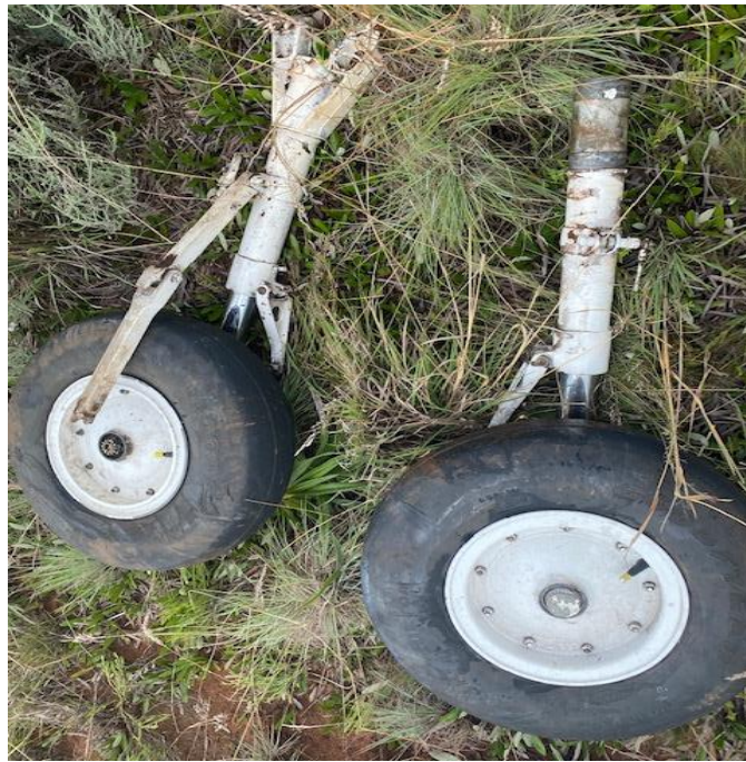
Figure 8: View of the broken main landing gear struts with the wheel assemblies still attached.
