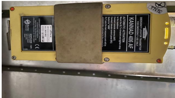
Figure 15: The ELT as installed on the aircraft's tail-section.
