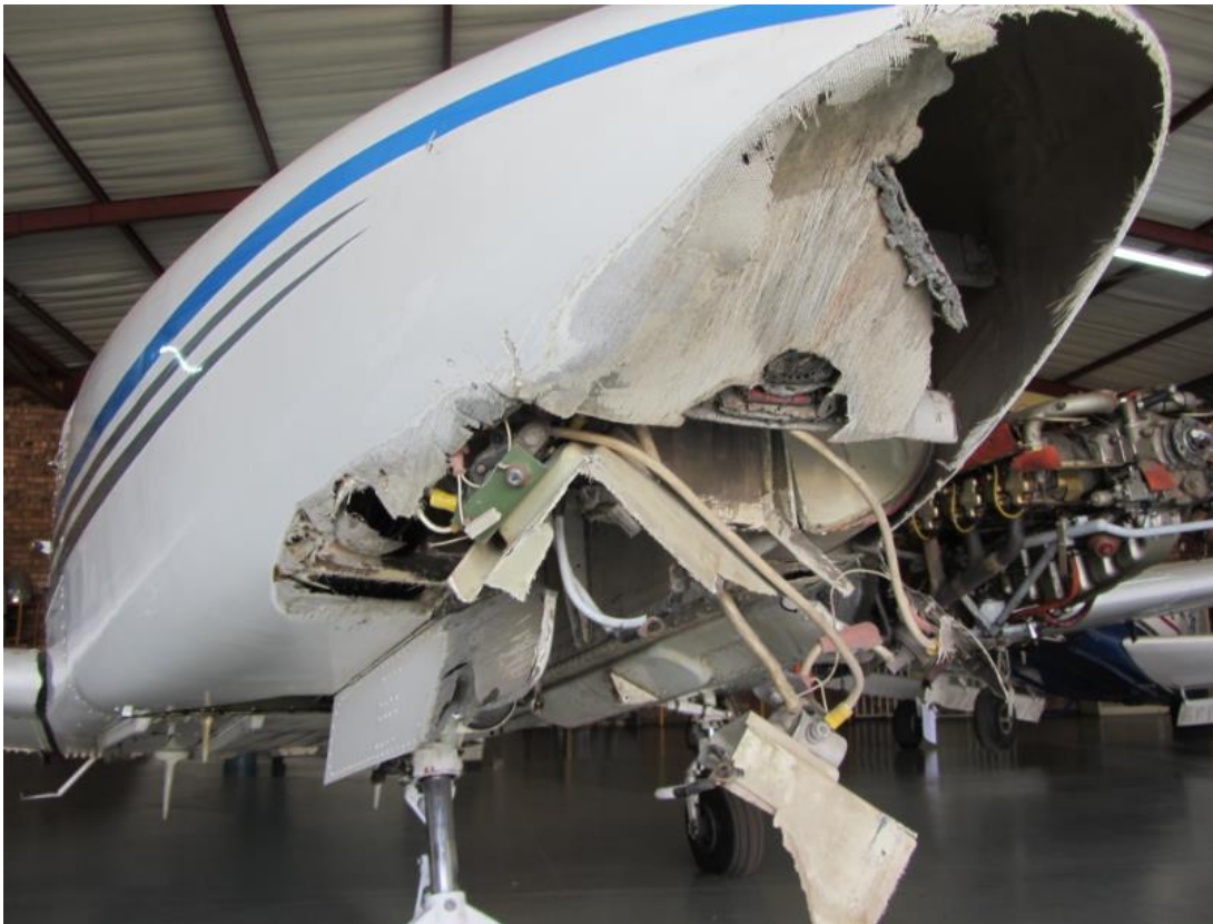
Figure 3: The damaged nose section.
