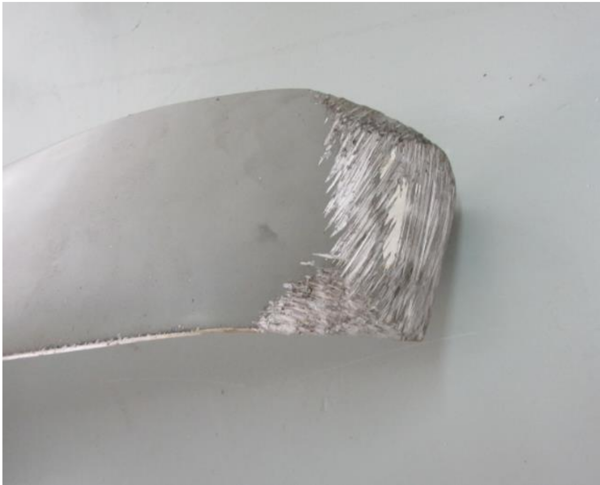
Figure 7: A propeller tip with scrape marks.
