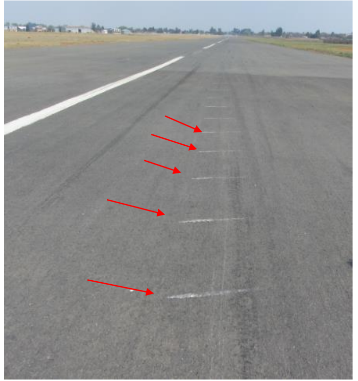
Figures 4 and 5: Arrows showing left- and right-side propeller tip marks on the asphalt runway.
