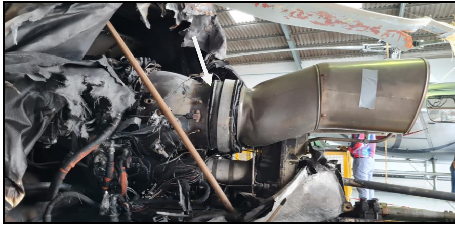
Figure 5: The engine compartment after fire damage.
