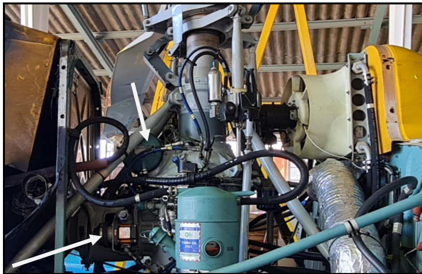
Figure 6: Hydraulic reservoir and pump found intact post-accident.
