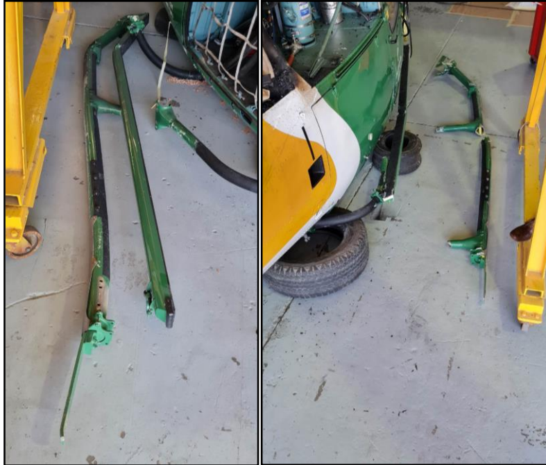
Figure 8: The left skid gear (left image) and the right skid gear (right image).
