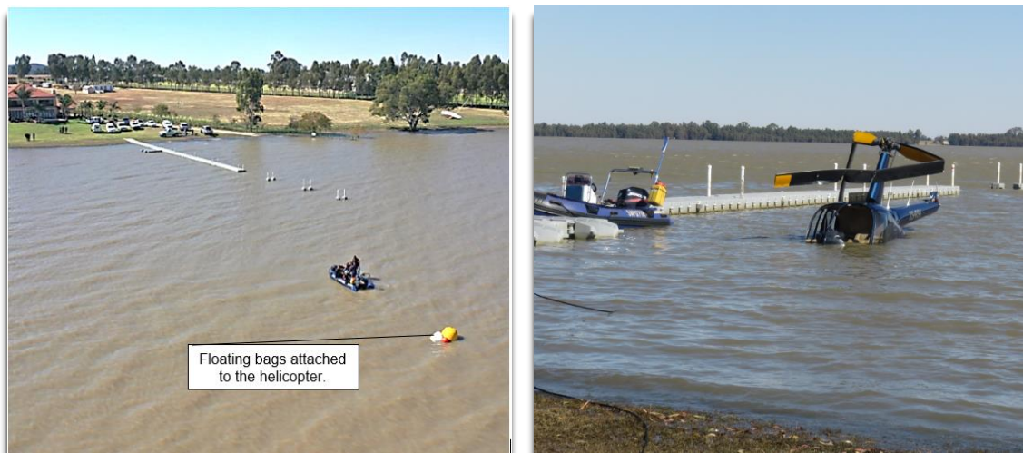
Figure 4: Left: Floating equipment attached to the helicopter; Right: The helicopter after being pulled ashore by the rescue boat.
