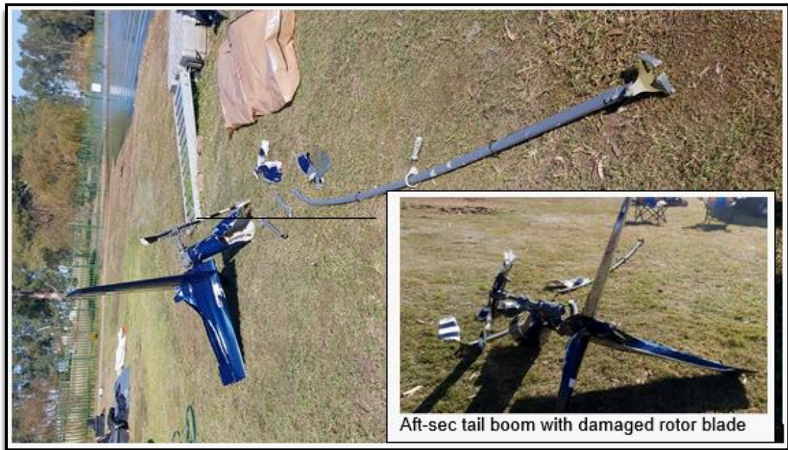
Figure 11: The aft-tail boom section, damaged tail rotor and the drive shaft.
