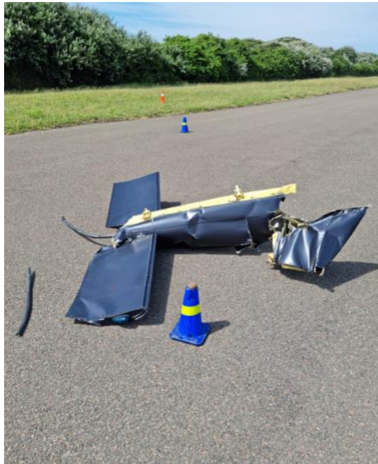
Figure 7: Horizontal stabiliser and control tube. (Source: Ronald Collyer)
