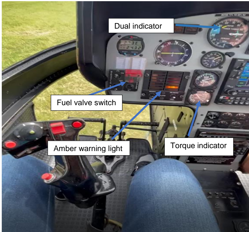
Figure 2: Arrows indicate positions of the fuel valve, torque indicator and dual gauge. (Source: Video footage from the passenger)
