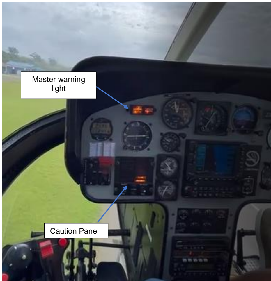
Figure 3: Master warning and caution as well as an additional caution message on the panel. (Source: Video footage from the passenger)
