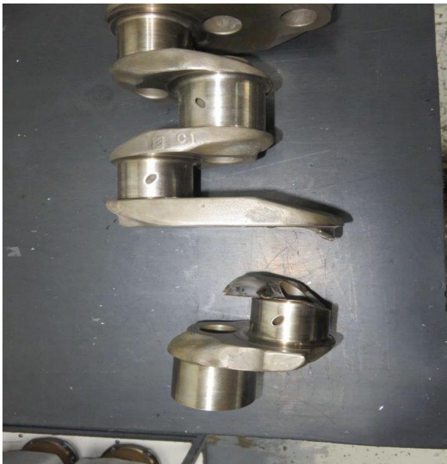
Figure 2: The crankshaft showing the area where the failure occurred.
