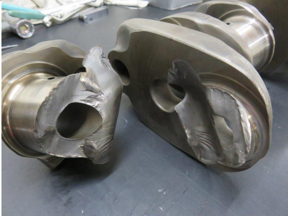
Figure 3: A closer view of the crankshaft showing the area where the failure occurred.
