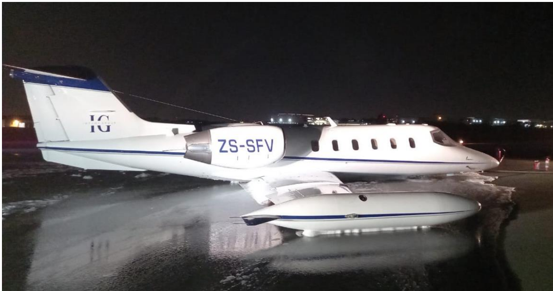
Figure 7: The ZS-SFV aircraft as it came to rest on its belly on the runway. (Source: AMO)
