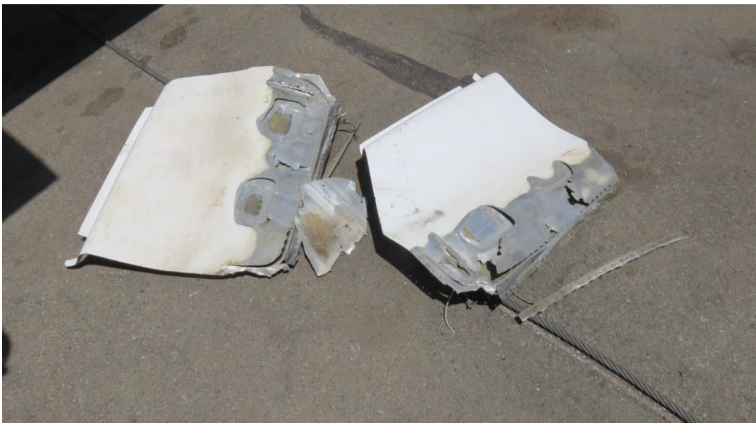
Figure 10: Damaged main landing gear doors.
