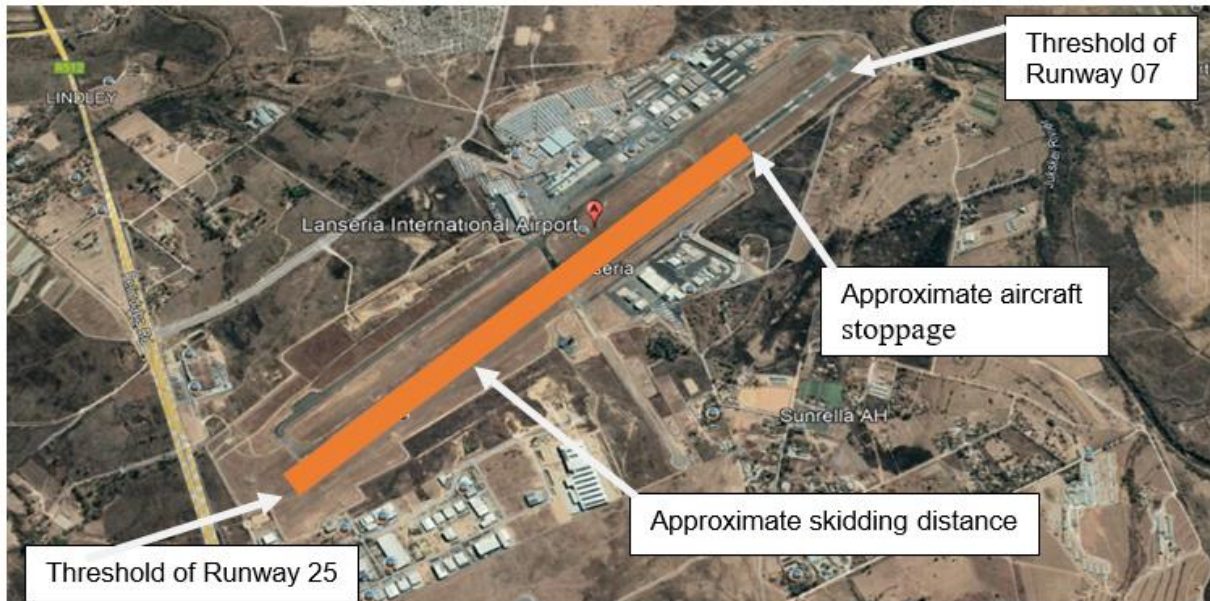
Figure 3: The approximate skidding distance of the aircraft during the accident. (Source: Google Earth).
