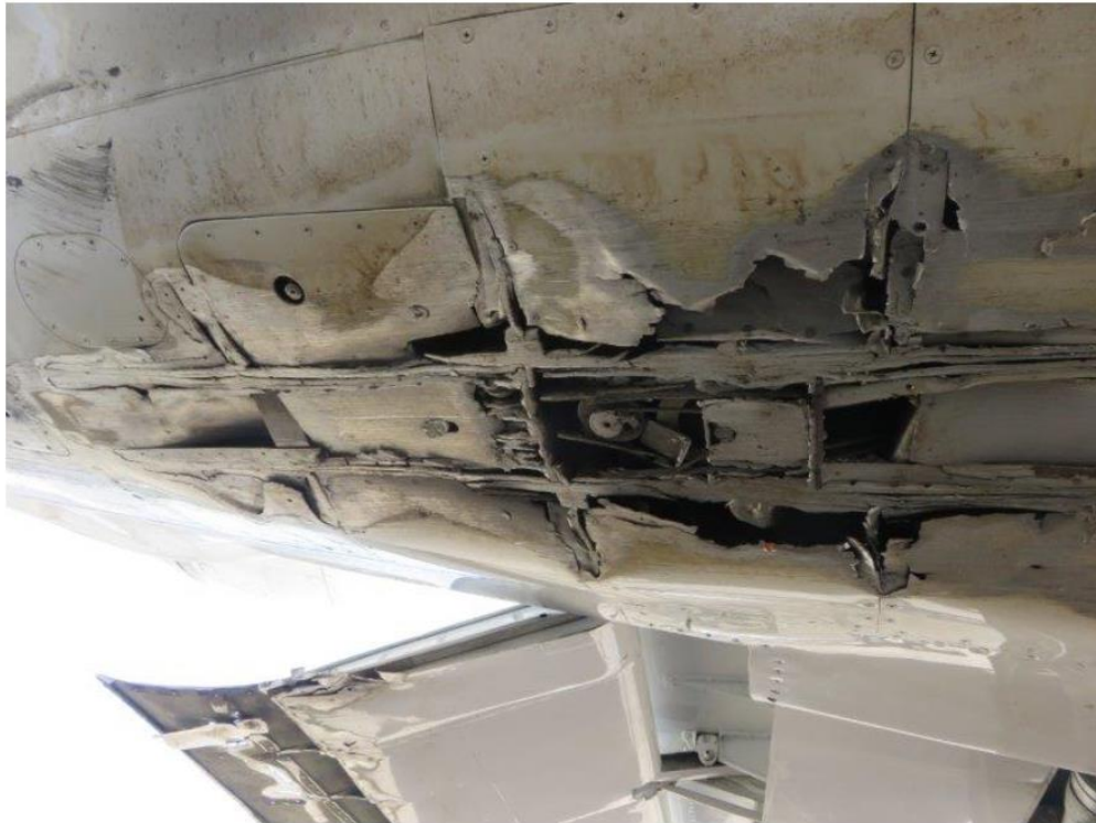
Figure 4: The damage underbelly and flaps.
