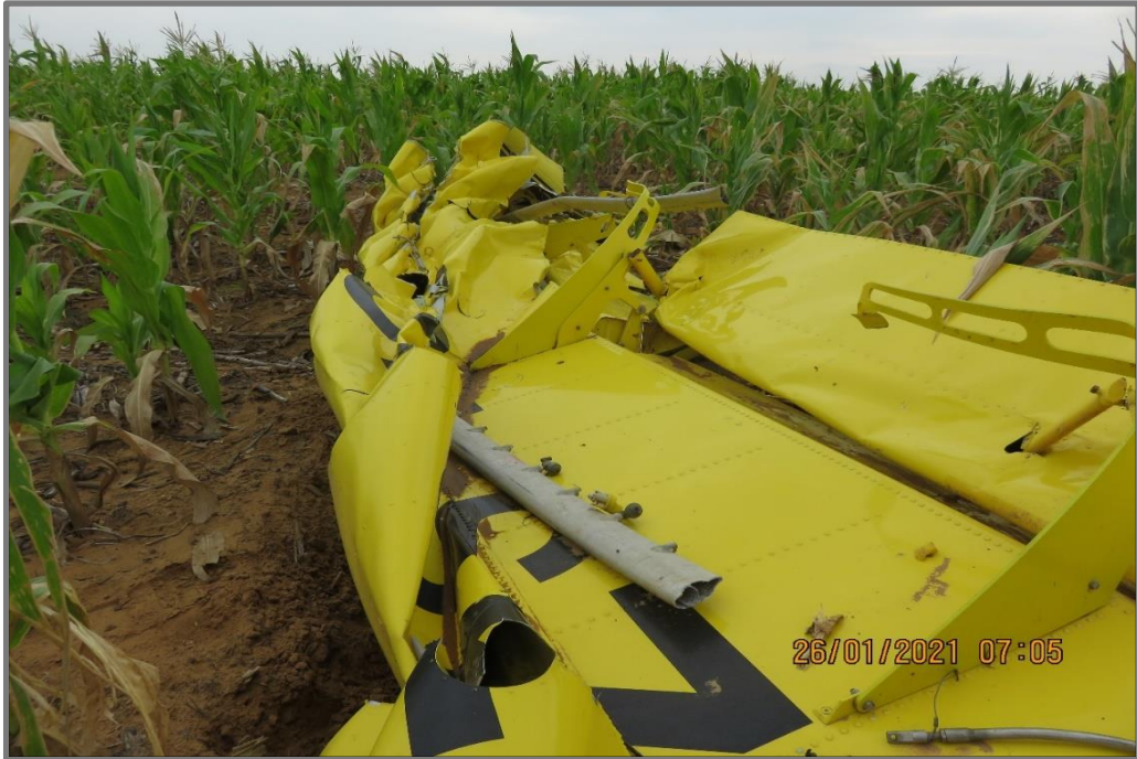
Figure 5: The damaged left wing due to impact.
