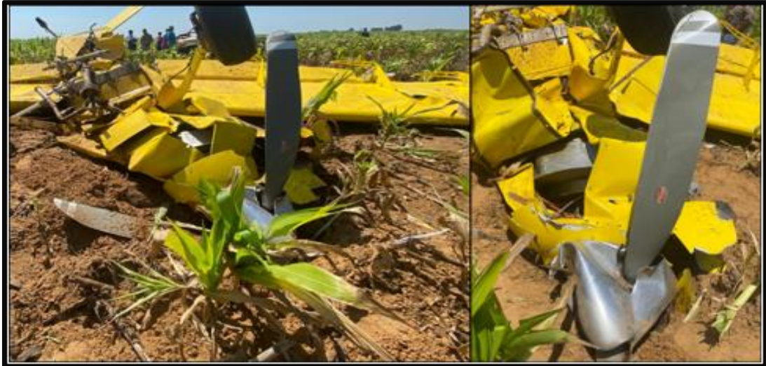
Figure 6: The damaged propeller.
