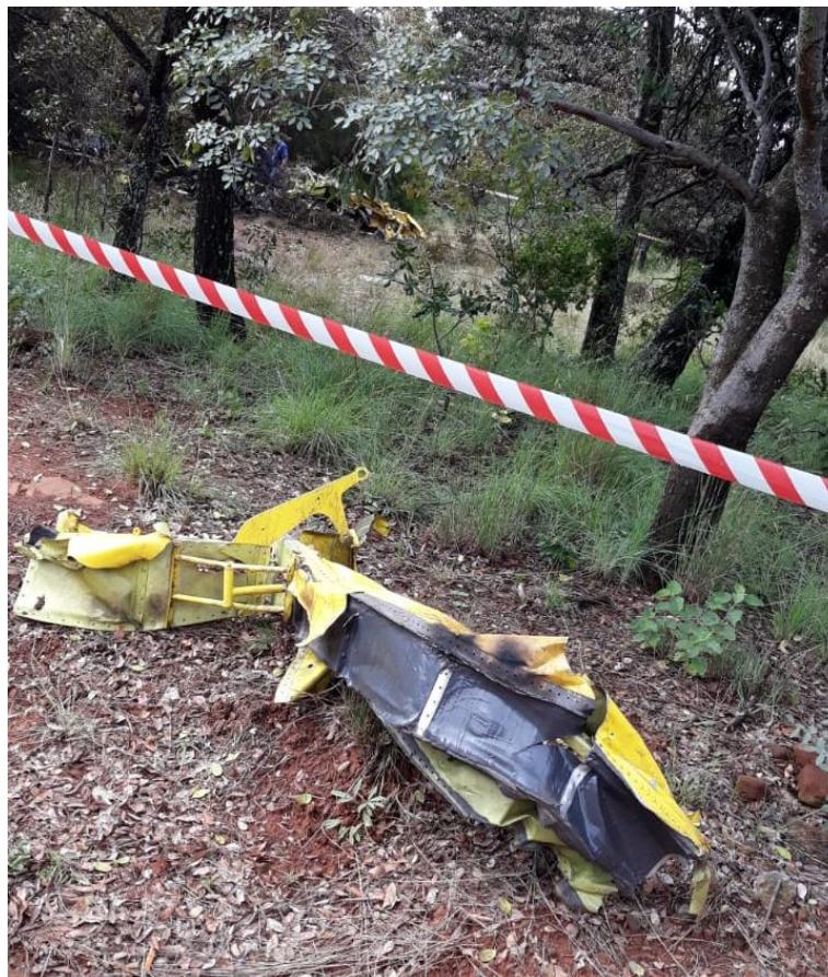
Figure 10: The left-wing aileron attachment.
