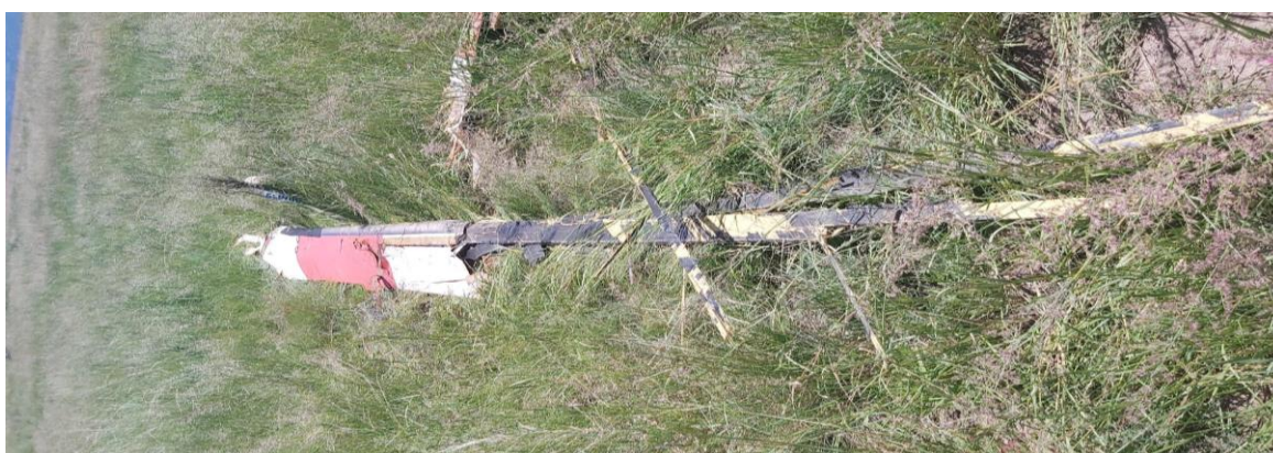
Figure 12: Orange main rotor blade landed 94m from the tail boom.
