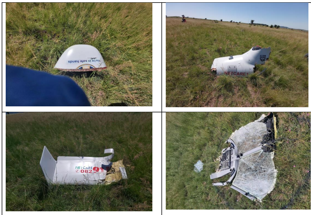
Figures 8, 9, 10, 11: Some helicopter parts that broke off in-flight before impact.
