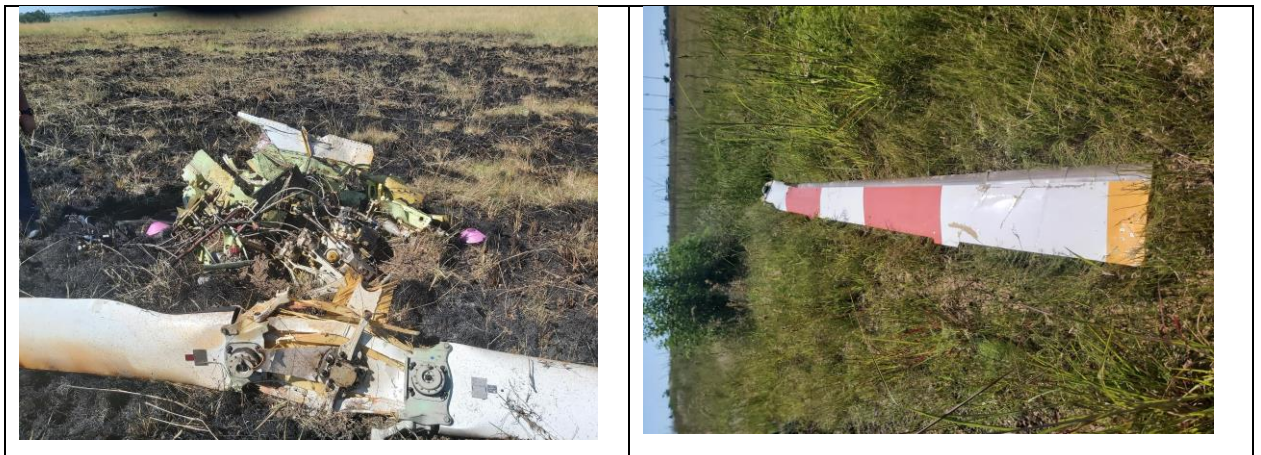
Figure 17: The gearbox that was not consumed by fire. Figure 18: The green main rotor blade.
