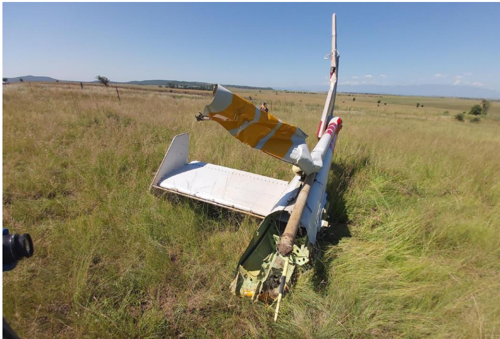
Figure 15: The tail boom was located 129.9m from the main wreckage.
