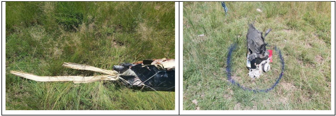
Figures 13, 14: The root of orange blade separated from the blade before impacting the ground.
