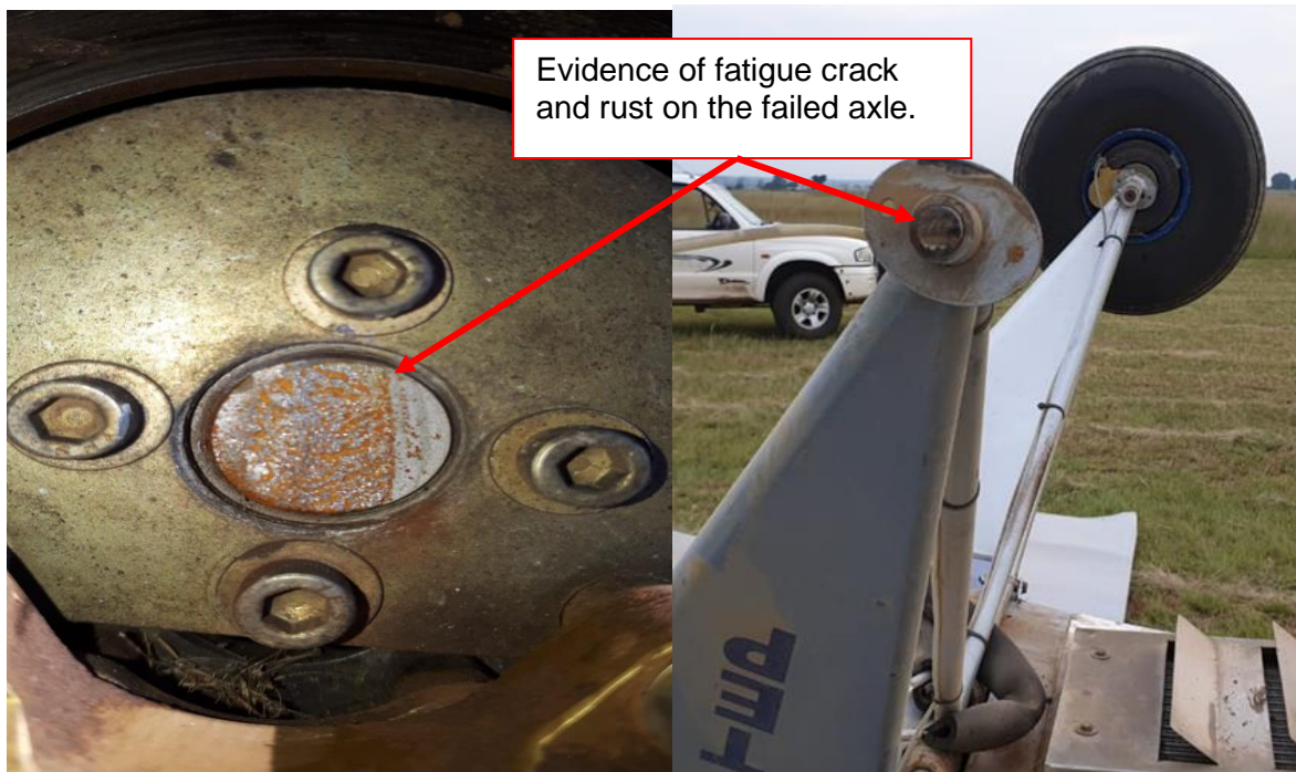
Figure 3 and 4: Close view of the failed axle
