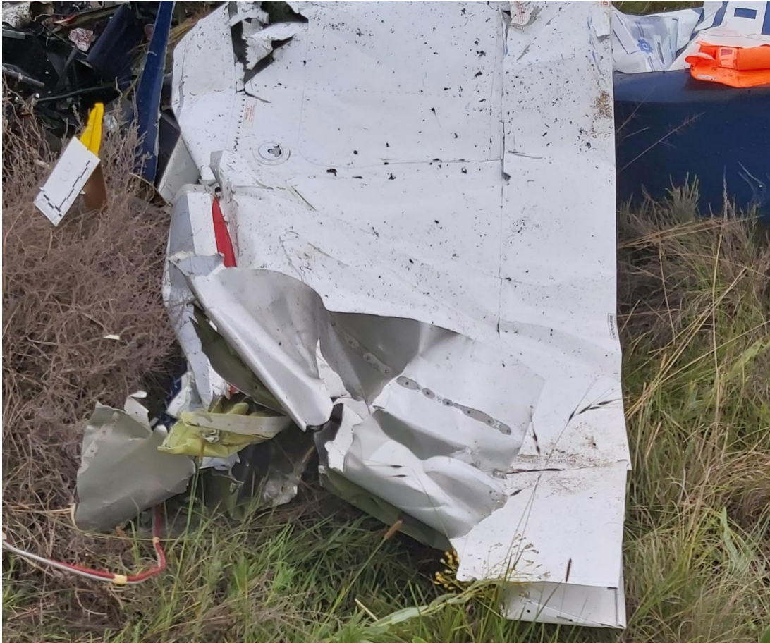
Figure 12: The left wing, which was found still attached to the main wreckage.
