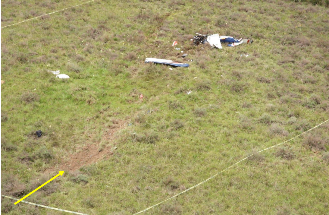
Figure 10: An Aerial photograph of the impact point, the right wing and the main wreckage.
