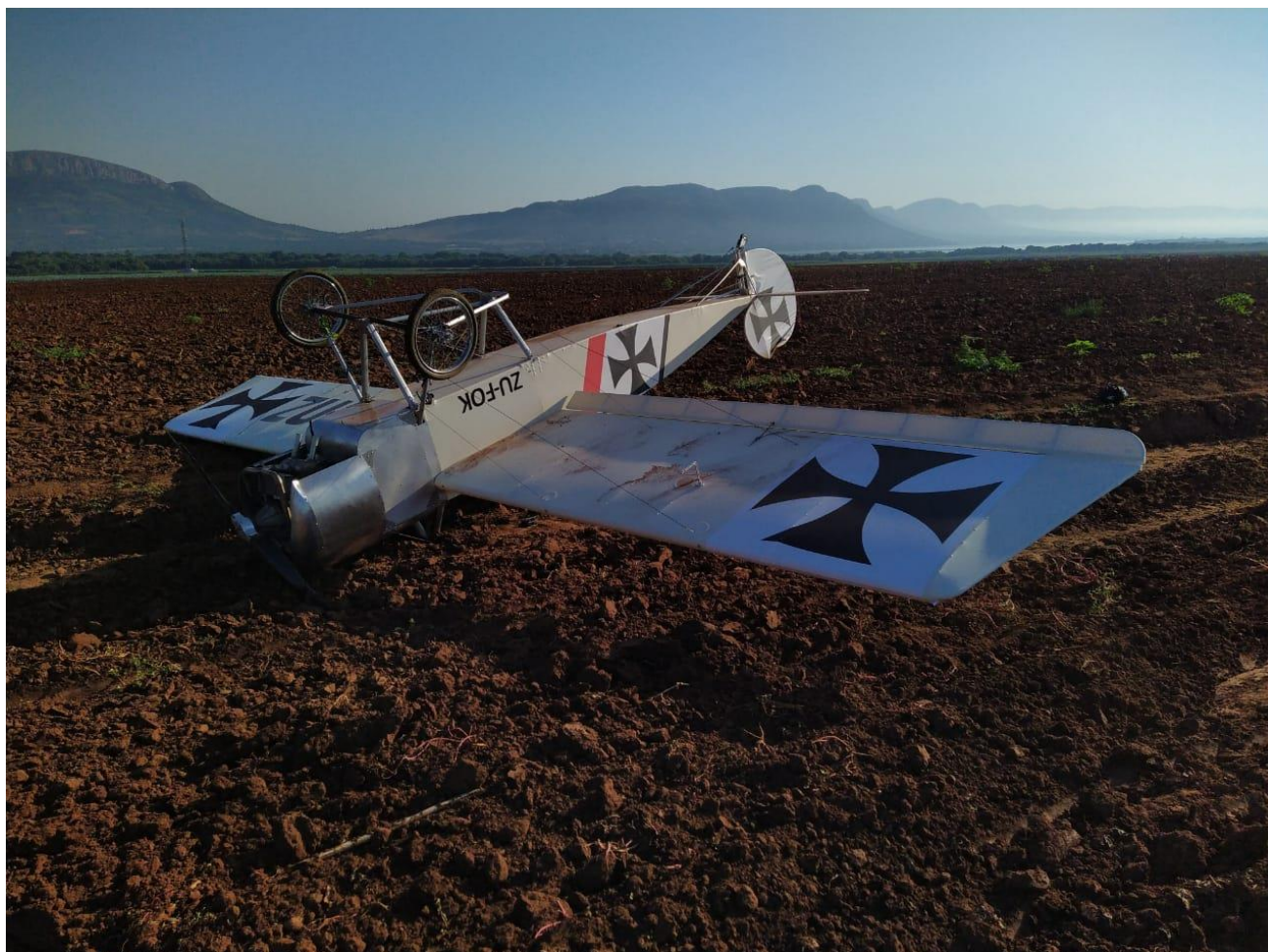
Figure 3: The aircraft with damage to the wing. (Source: pilot)
