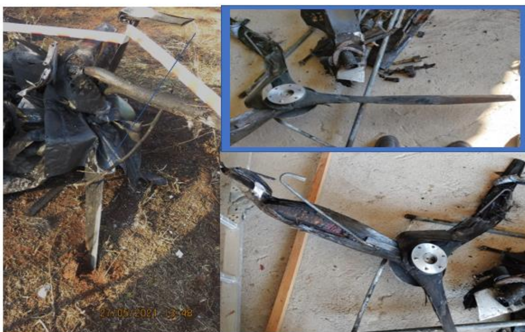
Figure 7: The damage on the propeller blades.
