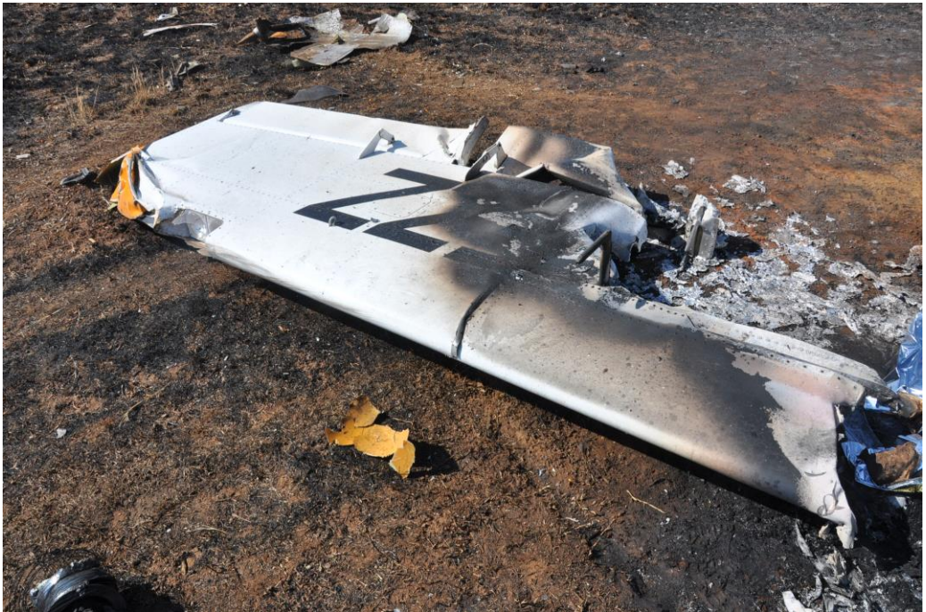
Figure 12: The left-wing that made contact with the ground first shows signs of impact damage on the wing tip.
