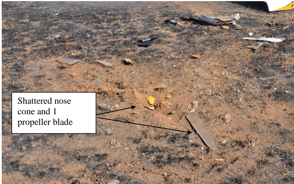
Figure 13: The second ground scar caused by the engine propeller blades.
