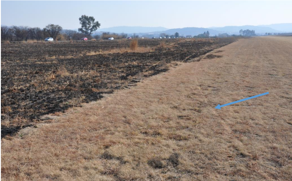
Figure 9: The first ground scar shows that the aircraft had veered off to the left after touchdown before taking power for next circuit.
