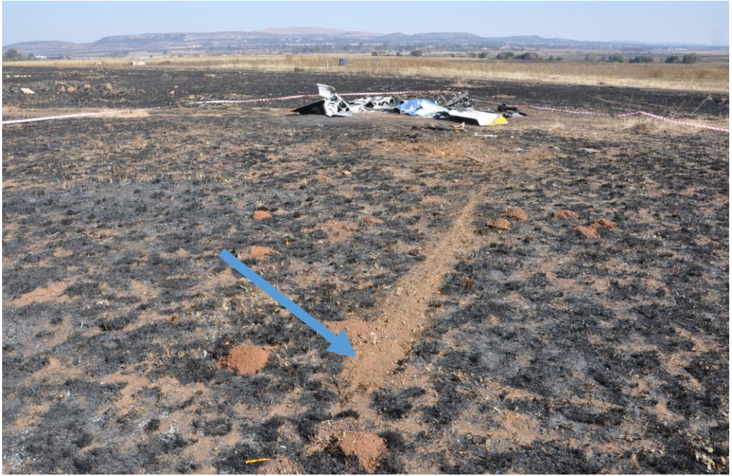
Figure 11: The first ground scar made by the left wing.
