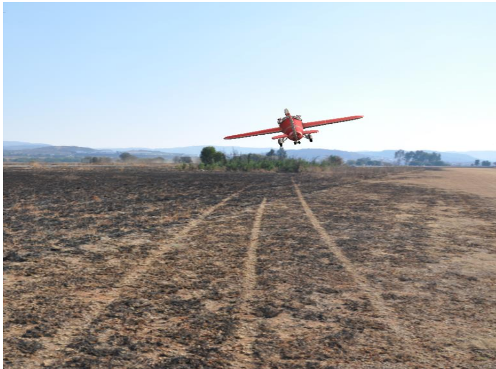
Figure 10: The second ground scars show the aircraft rolling before lift-off, with the student pilot attempting to avoid collision with the trees. (Aircraft figure source: 3D library)
