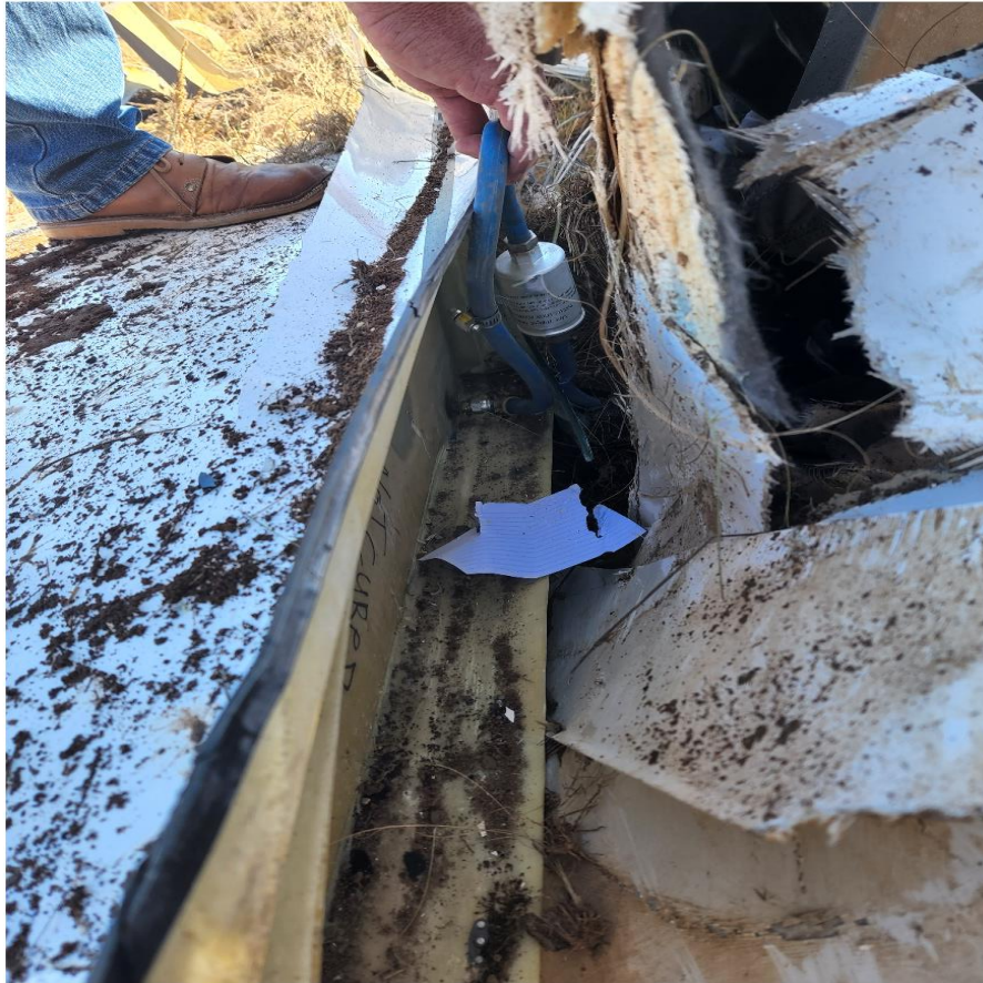
Figure 7: The separated wing from the root.
