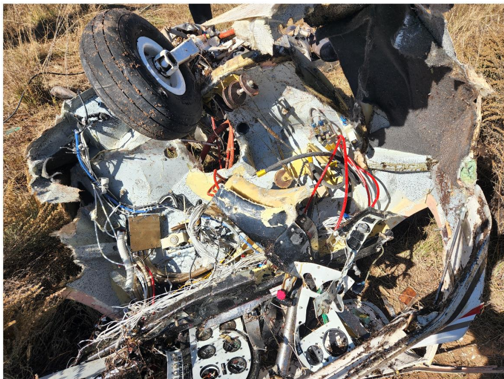
Figure 10: The destroyed instrument panel and the nose gear in the cockpit.
