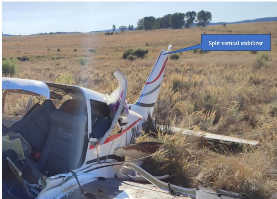
Figure 9: The split vertical stabiliser.
