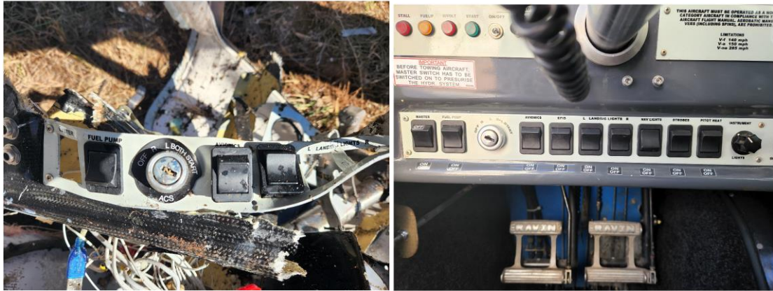
Figure 11 and 12: Position of the switches after the accident (left); and the position of switches in a stationary aircraft that is similar to the accident aircraft (right).
