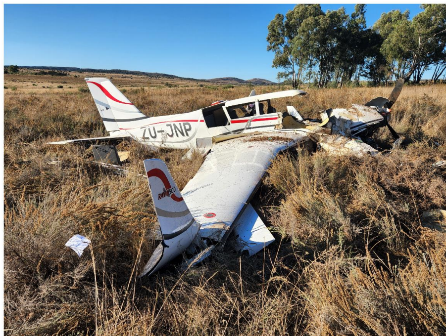
Figure 6: Damage on the right-wing tip.
