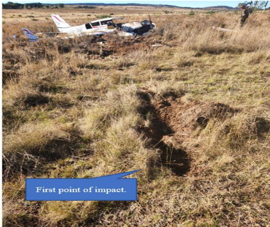
Figure 5: The first point of impact and the aircraft's resting position.
