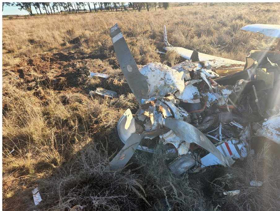
Figure 8: The damaged spinner and the propeller blade.
