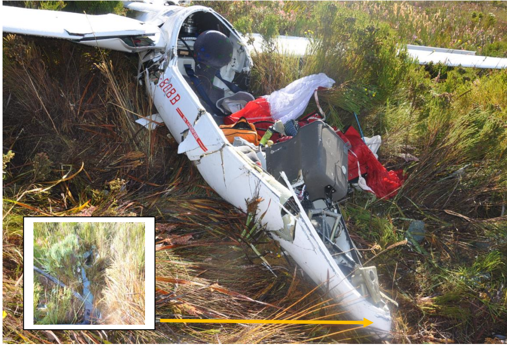
Figure 10: The damaged cabin section. The inset shows an indentation on the ground caused by the nose during impact.
