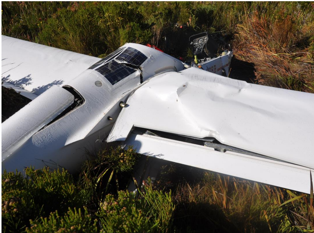
Figure 8: Buckling and deformation of the skin surface.
