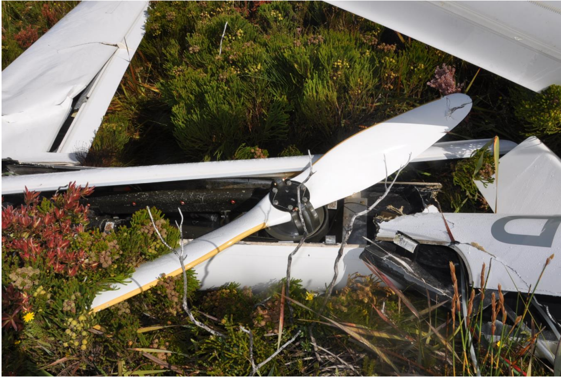
Figure 13: Propeller blades as found at the accident site.
