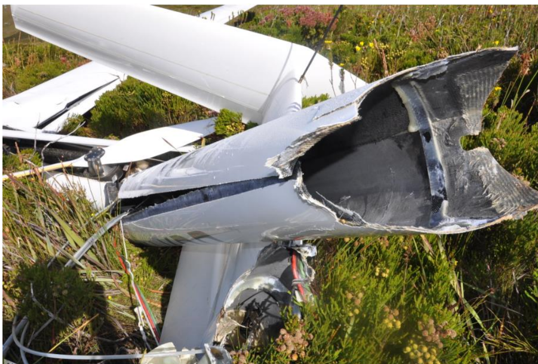
Figure 12: Damage sustained by the empennage.
