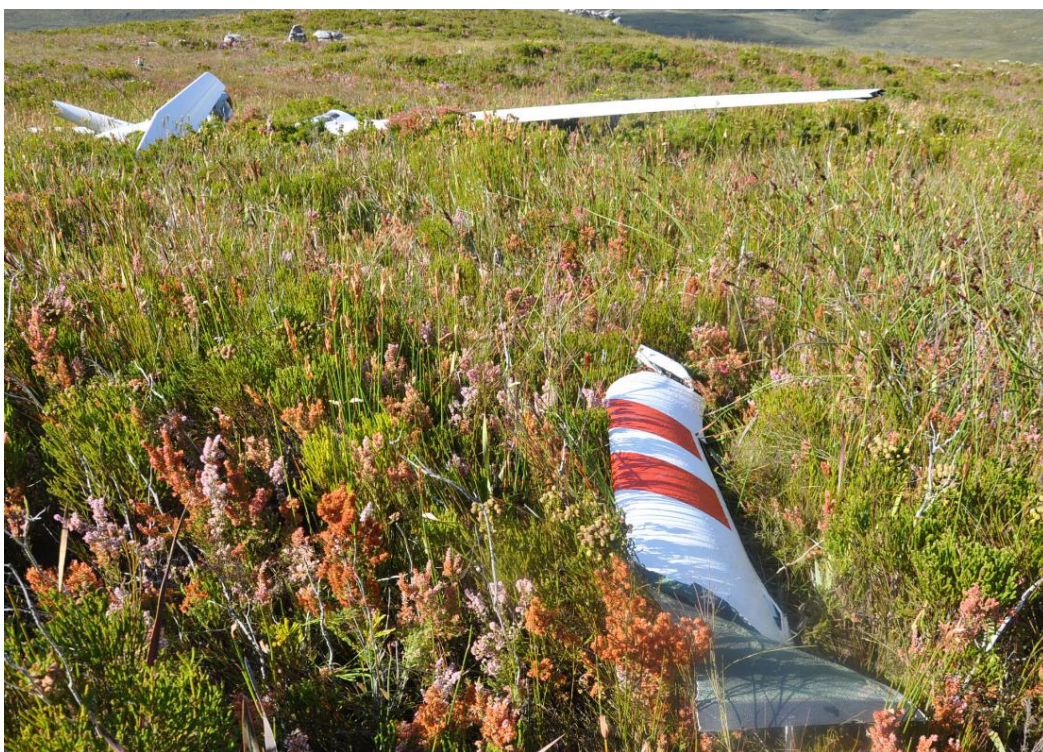
Figure 9: Detached right-side winglet.
