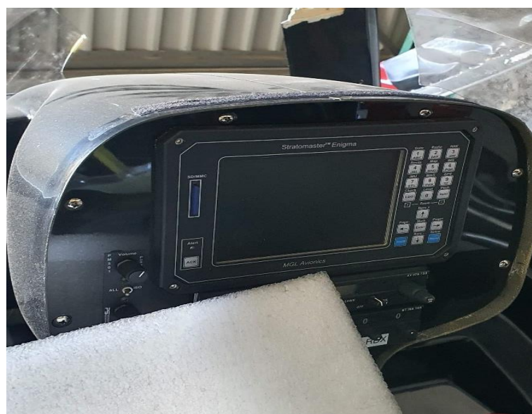
Figure 4: MGL Avionics Stratomaster Enigma installed in the helicopter.
