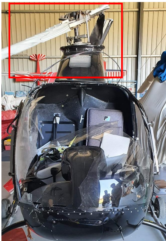
Figure 8: The red block shows the condition of the main rotor hub assembly and rotor blades post-accident.
