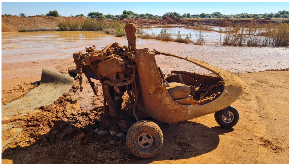
Figure 2: The gyrocopter after the eyewitnesses had moved it to stable ground.
