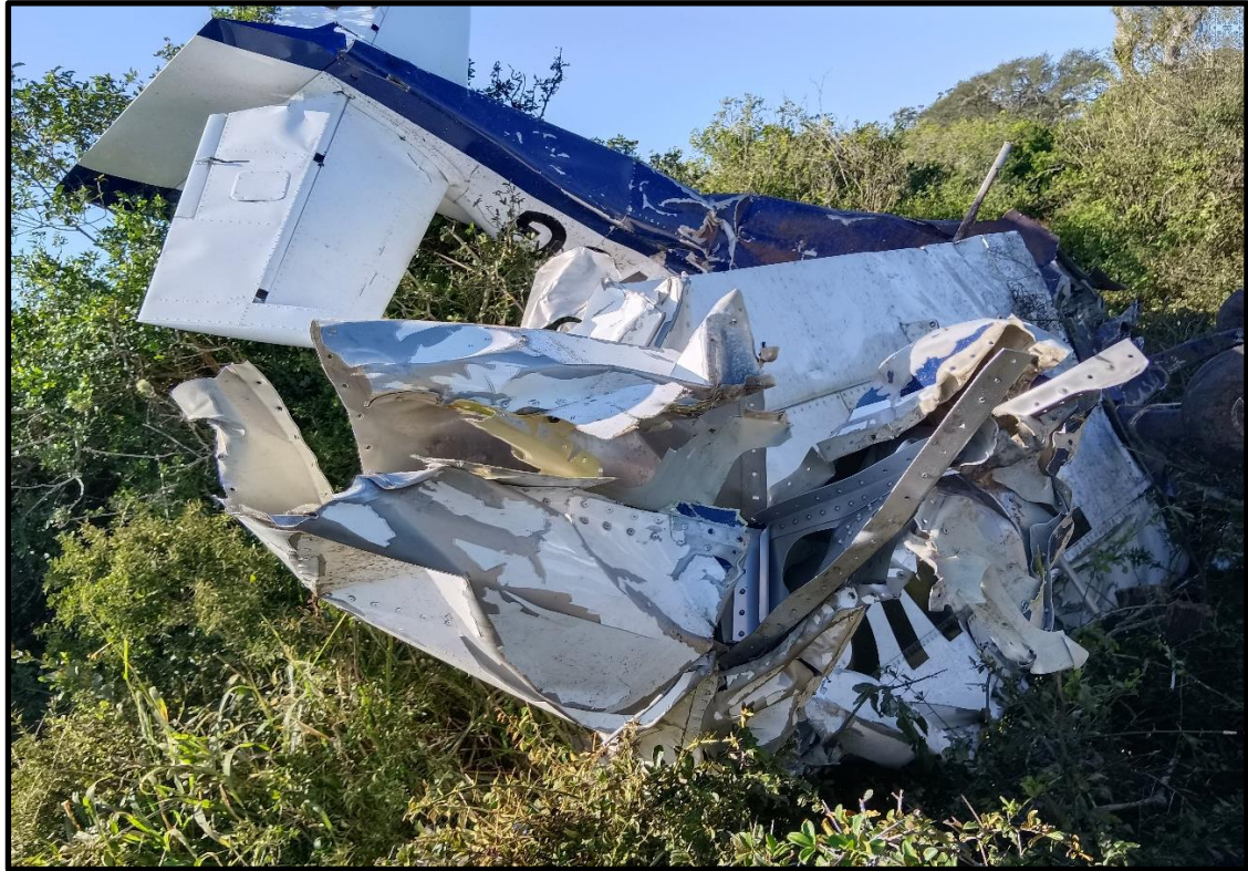
Figure 9: Damage on the outer part of the left-side wing.
