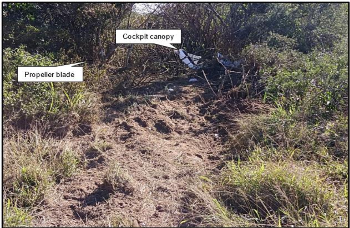
Figure 5: The second impact point as well as some cockpit debris.
