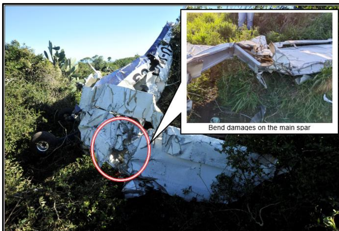
Figure 8: The damage on the right-side wing.
