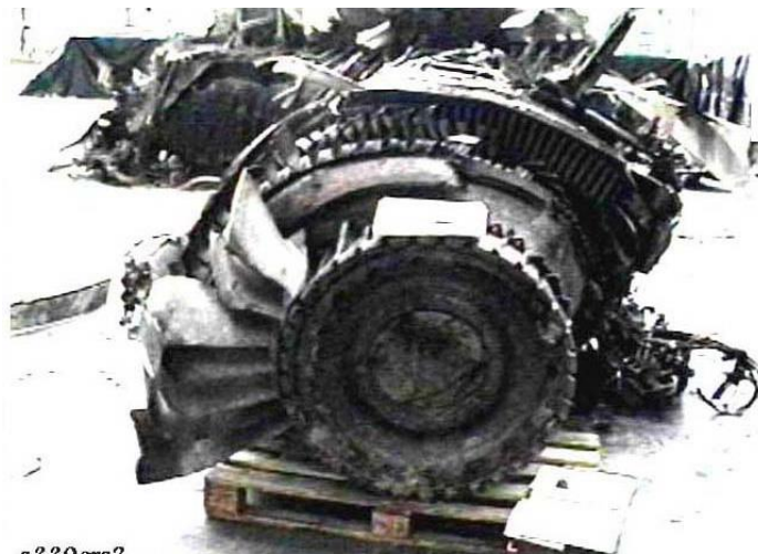
Figure 4. High speed damage
