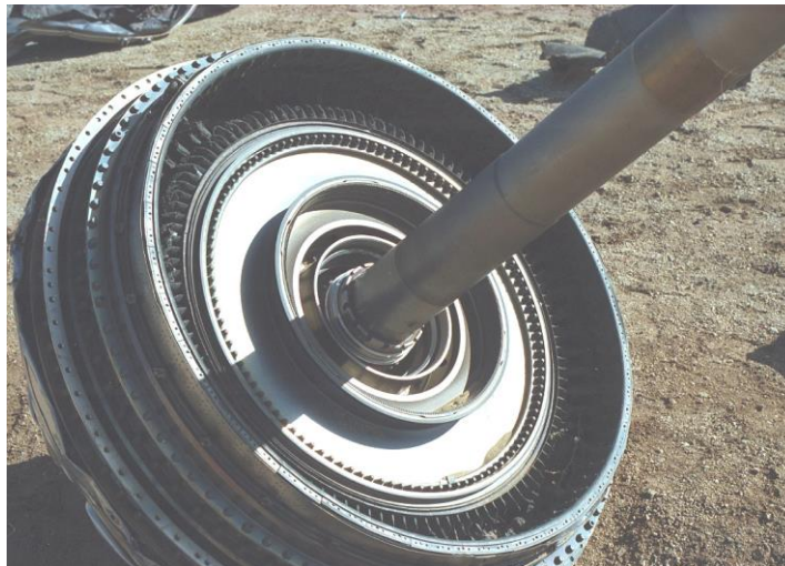
Figure 2 This photograph illustrates the problem of taking photographs on a clear day with bright sunlight as the only illumination. It was made to illustrate heat damage to the turbine section. Note that most of the detail of the damage is lost in the shadows.
