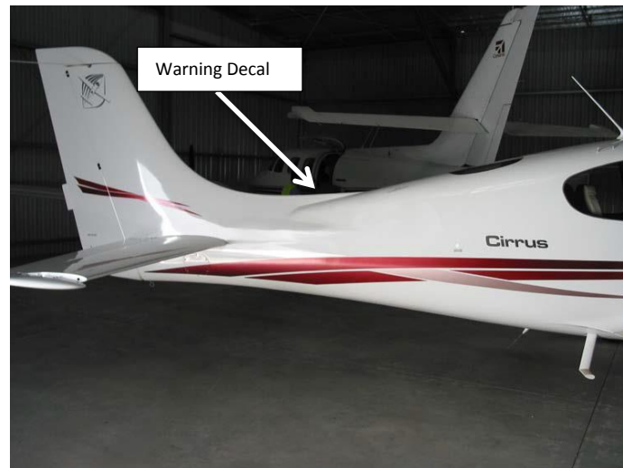
Figure 13. Side view of rear of Cirrus aircraft highlighting the CAPS warning decals on fuselage
