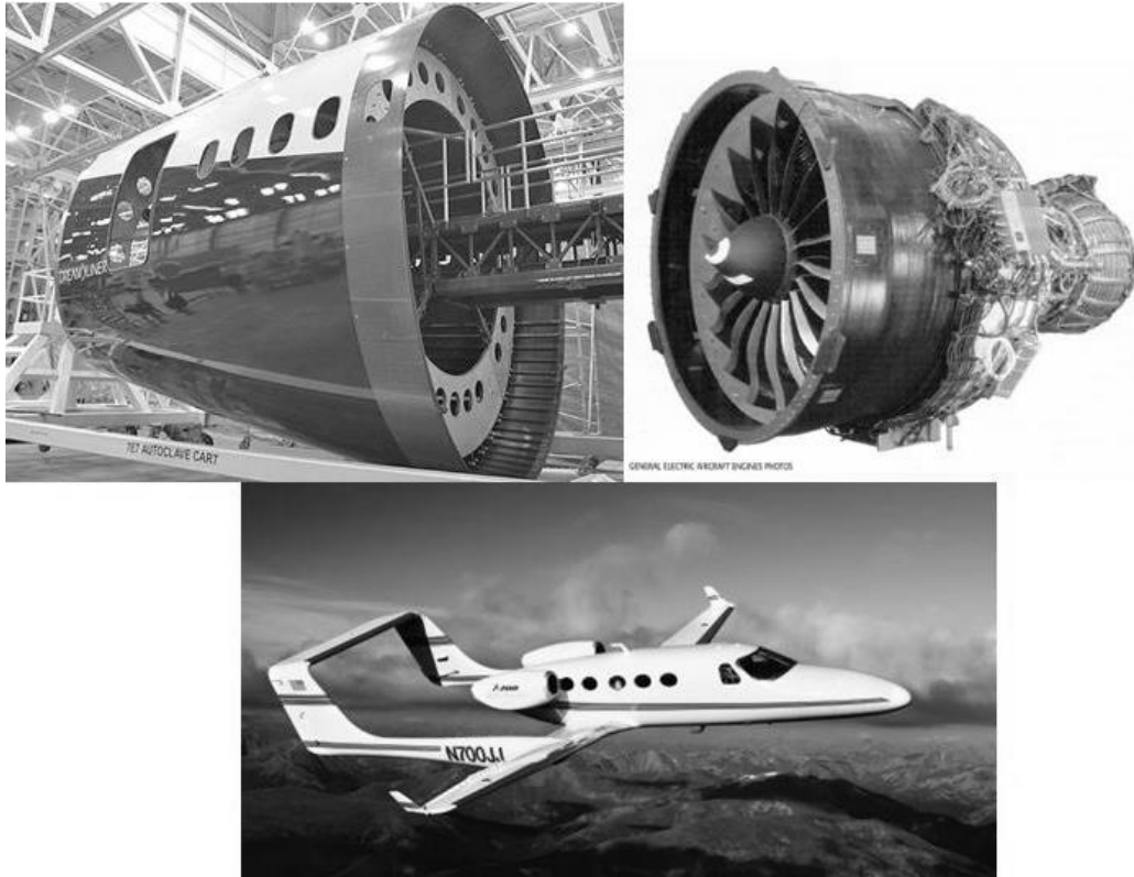
Figure 21. Examples of composite structures (clockwise from top): Boeing 787 fuselage, General Electric GENx fan blades and case, Adam Aircraft A700 VLJ.
