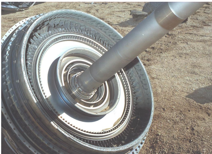
Figure 3. This photograph was made using a flash attachment powerful enough to illuminate the shadowed areas of the photograph on a clear day under full midday sun. The damage to the engine turbine section is clearly visible.
