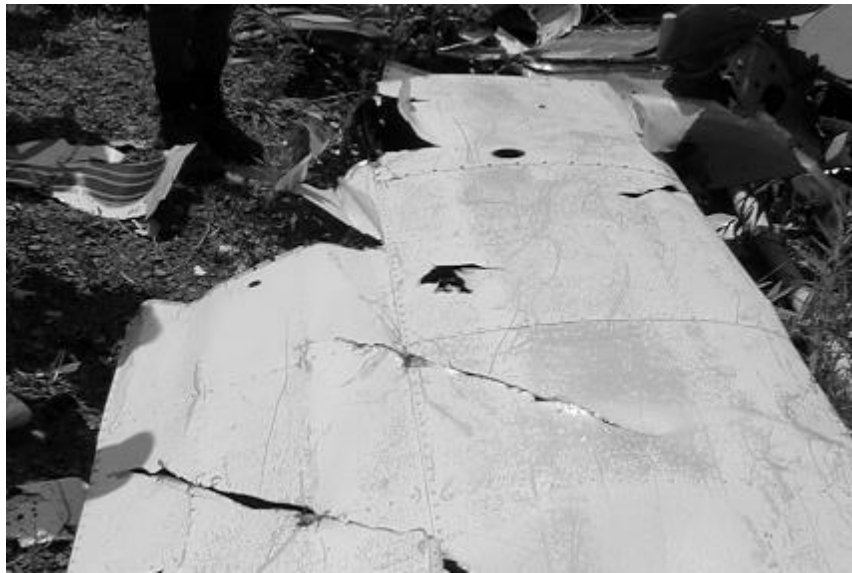
Figure 11. Connecting the mid points of multiple prop slashes will form an equivalent scratch mark.
