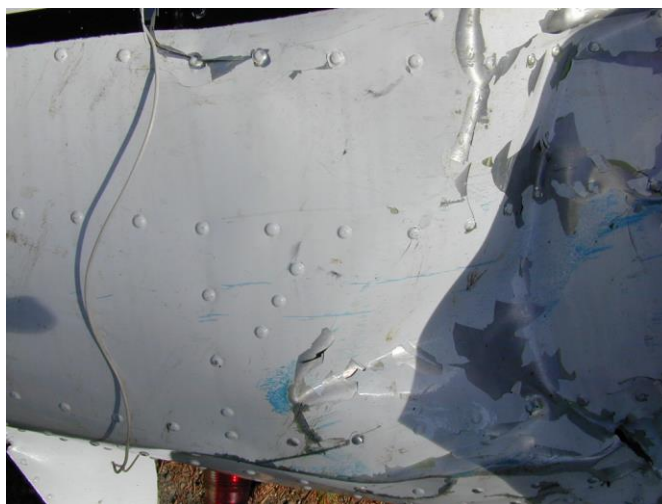
Figure 4. A vertical surface of a fuselage photographed from the side. Note the straight scratch marks and the relatively small angle formed with the longitudinal axis, showing little relative vertical movement in this collision.
