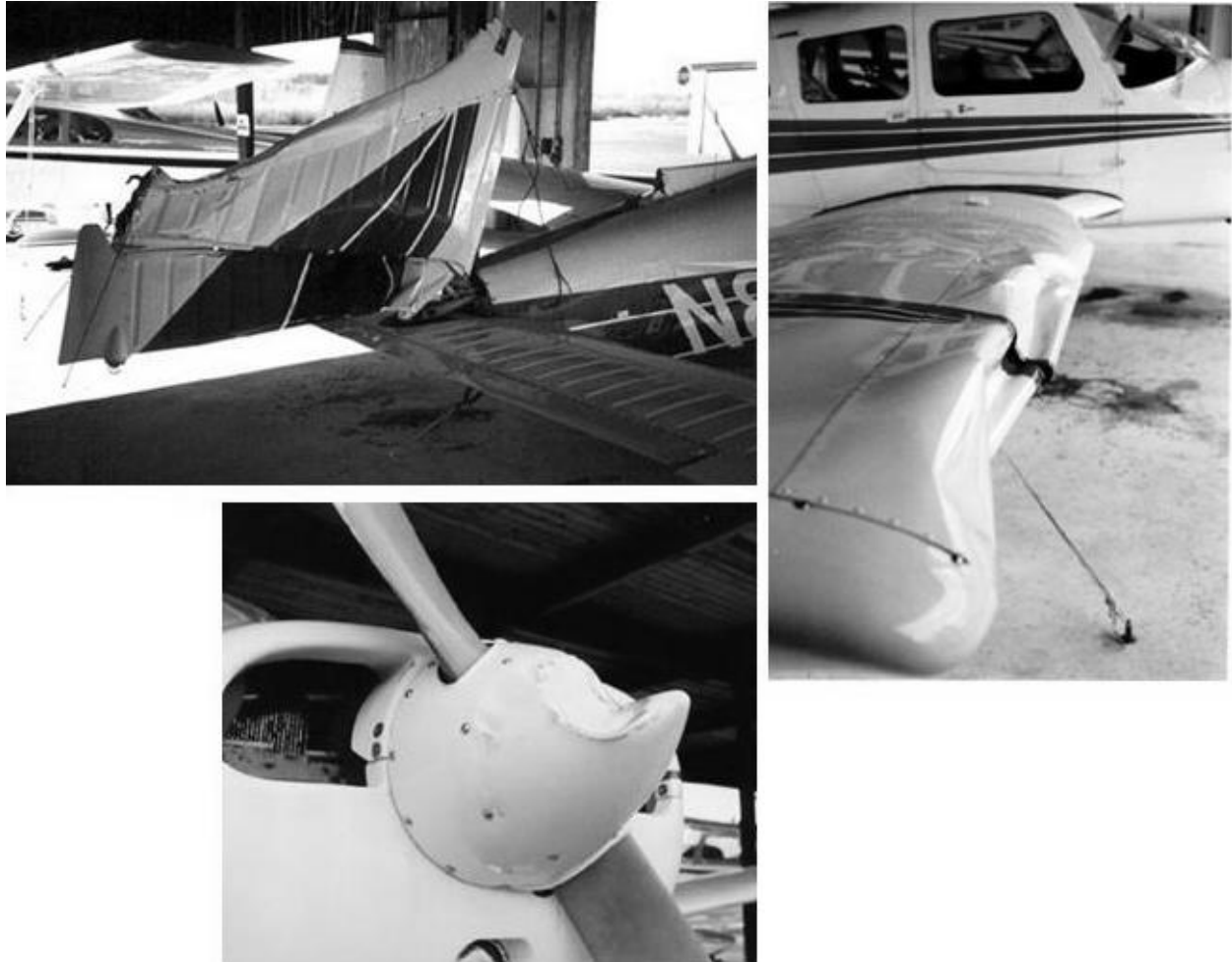
Figure 24 The ductility of metal structures provides macrostructurally visible information regarding an accident.
