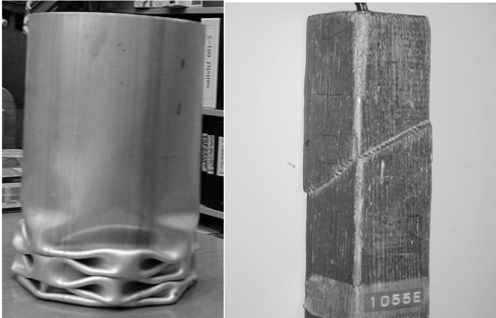
Figure 9. Compression (buckling) failure (left); Block compression failure (right)
