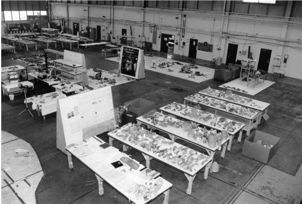
Figure 3. Systems Reconstruction Layout of Swissair 111 (Courtesy of Transportation Safety Board of Canada)
