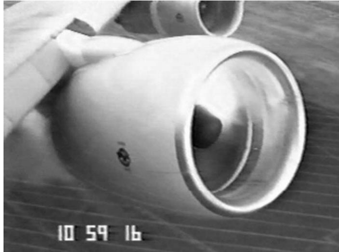
Figure 10. Flame out inlet and tailpipe in an engine stall/surge
