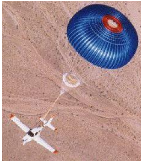
Figure 11. Rocket-deployed emergency parachute system
