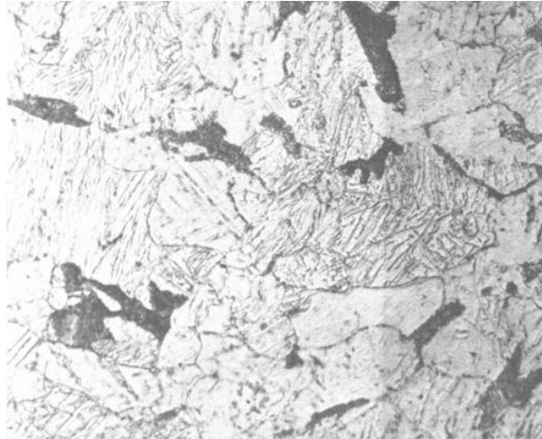
Figure 8. Crystal twinning in mild steel
