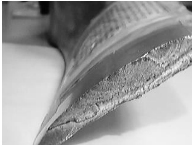
Figure 37. Propeller showing beach rings as a result of resonance fatigue failure
