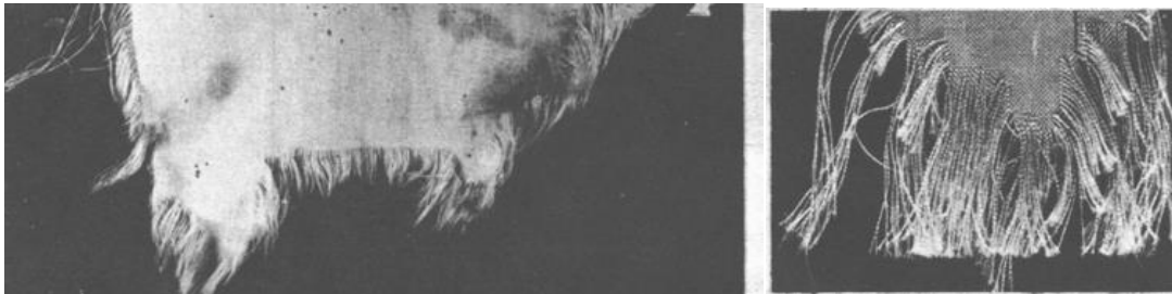
Figure 15. Teasing. Left: Fractured edges "fluffy" due to flapping in airstream. Right: Fracture after tearing.
