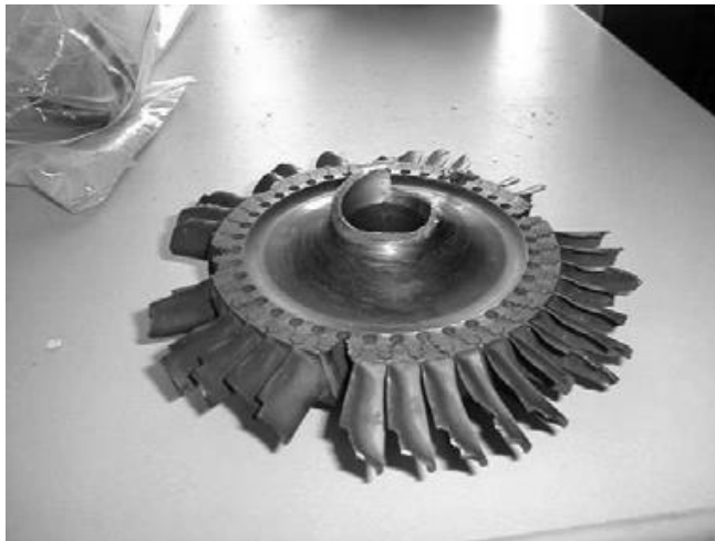
Figure 12. Torsion failures. Helicopter turbine (left); Turbine engine shaft failure (right)
