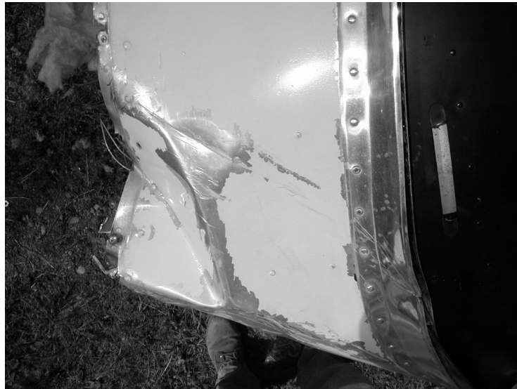
Figure 3. Scratch marks on a horizontal surface photographed from overhead. Note the straight lines.
