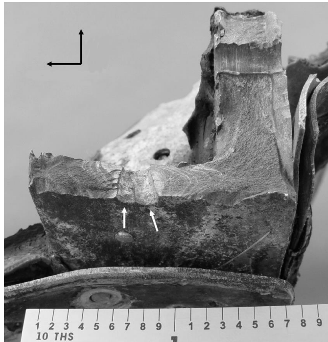
Figure 25. Indications of fatigue cracking in the lower right wing spar cap of the Chalks Ocean Airways Grumman Mallard G73 that crashed in December 2005. This is an example of using accumulated knowledge and experience with metallic structures to identify possible factors in an accident.
