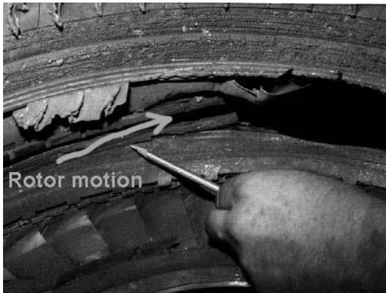
Figure 13. Squeeze-rupture penetration hole
