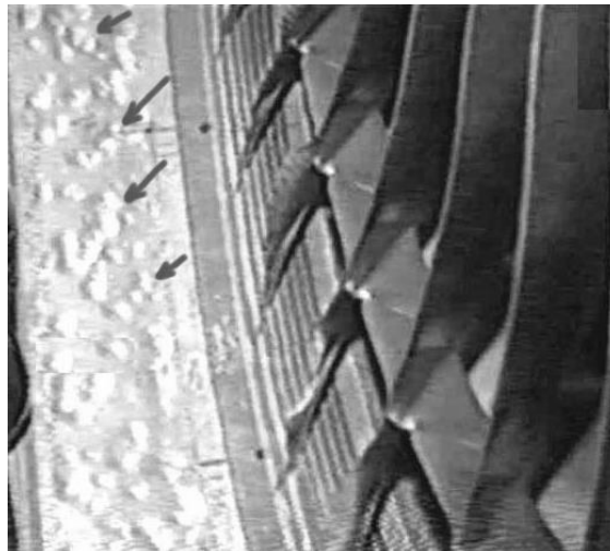
Figure 19. Dents in acoustic treatment due to ice released from fan rotor
