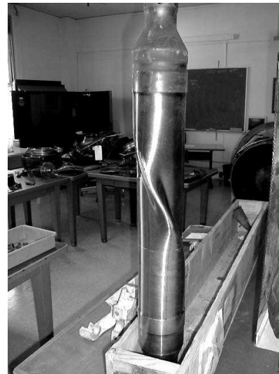
Figure 12. Torsion failures. Helicopter turbine (left); Turbine engine shaft failure (right)
