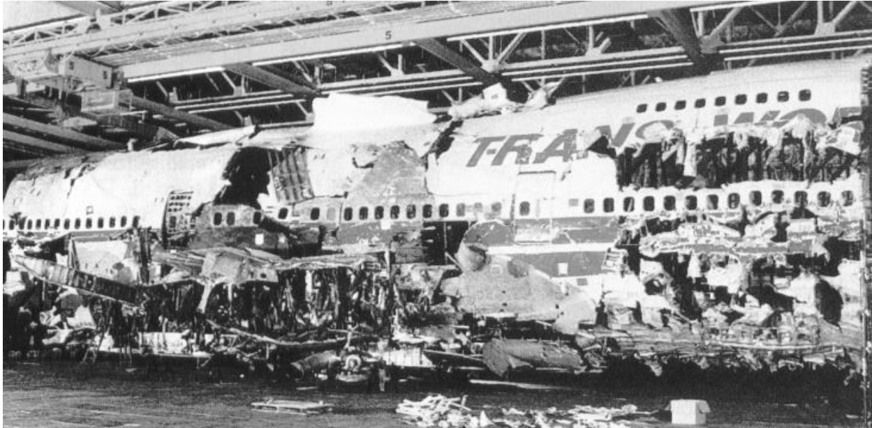
Figure 5. Reconstruction of TWA 800 main fuselage section (Courtesy of U.S. National Transportation Safety Board)
