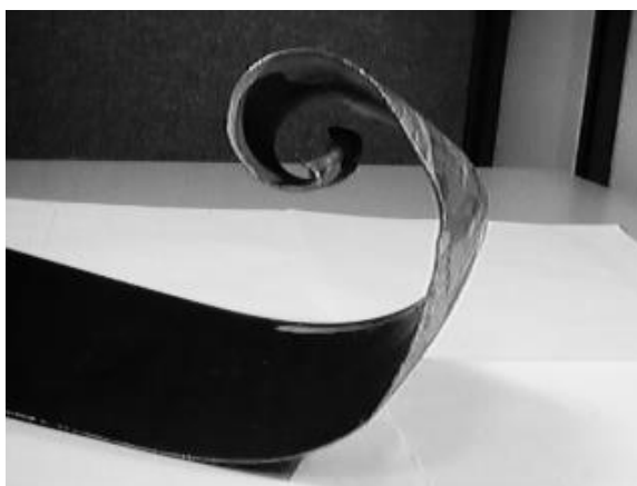
Figure 35. Propeller tip bent forward as a result of high rpm during a low-angle impact
