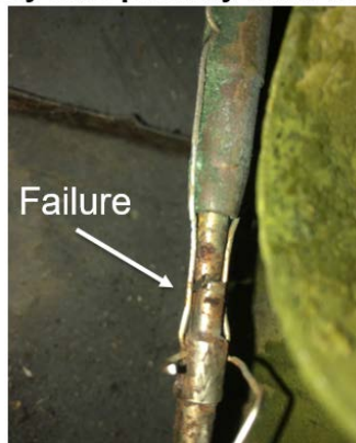
Right aileron control cable with safety wire partially removed
