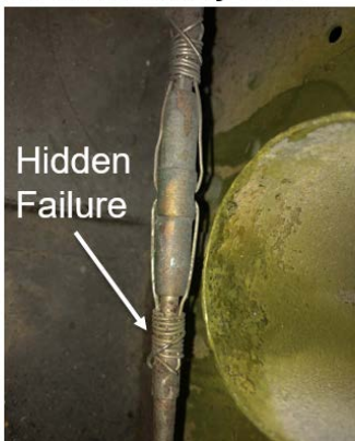
Right aileron control cable with failure under safety wire
