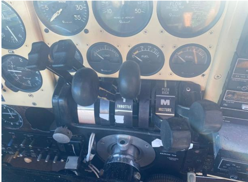
Figure 4: The throttle lever power quadrant after the accident. (Source: Operator)
