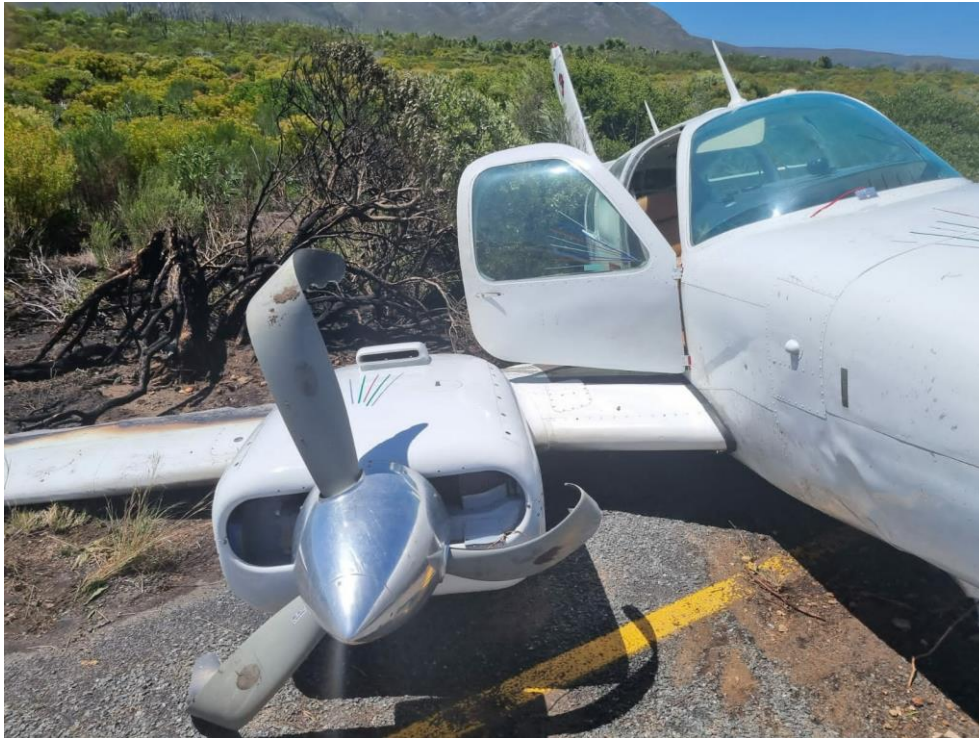
Figure 3: Damage to the right wing and propeller blades. (Source: Operator)
