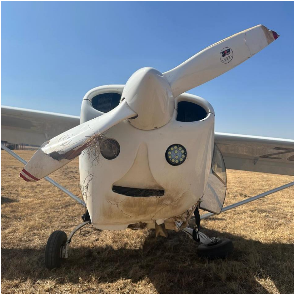
Figure 3: Damage to the propeller and the broken main left landing gear strut. (Source: Operator)
