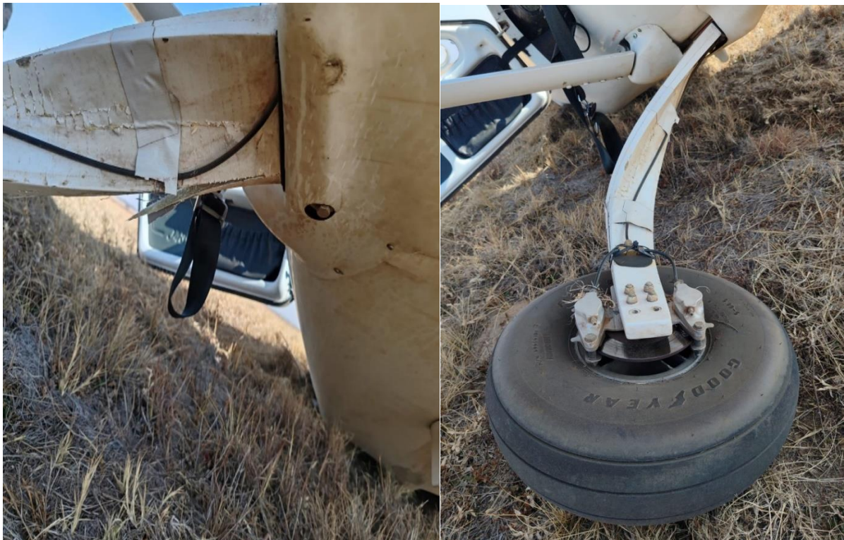
Figures 4 and 5: Delamination and damage to the left main gear. (Source: Operator)
