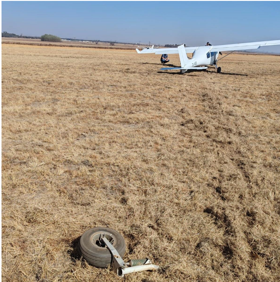
Figure 6: Damage to the landing gear. (Source: Operator)
