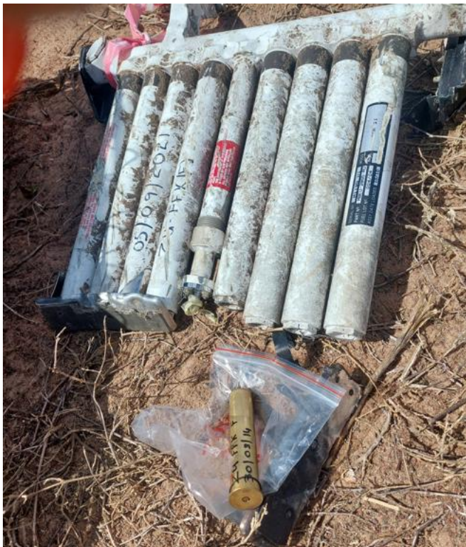
Figures 19 and 20: The rocket motor assembly which was not fired (left), and one that was fired (right).
