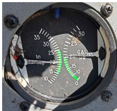
Figure 15: Manifold pressure and fuel flow dual indicator. (Source: Investigator)
