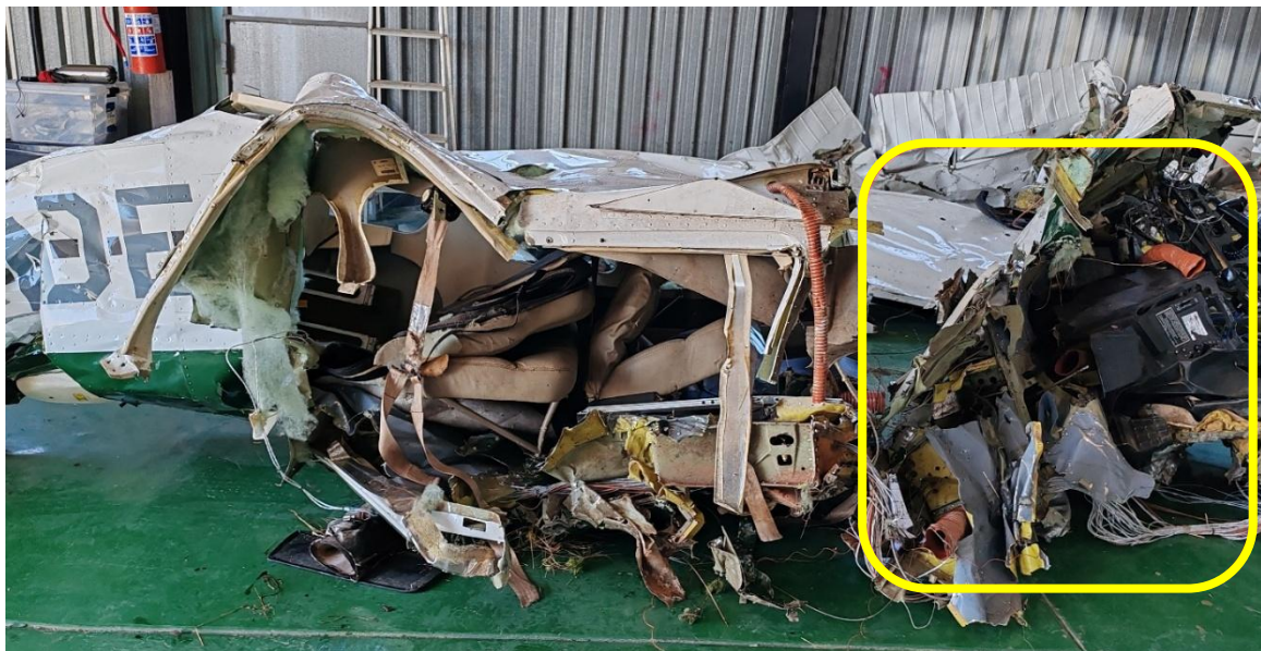
Figure 16: The cockpit was completely crushed during the accident sequence (yellow highlight). (Source: Investigator)
