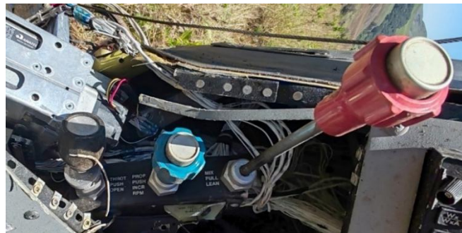
Figure 13: Throttle lever, propeller rpm lever and fuel mixture lever positions. (Source: Investigator)
