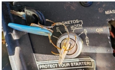
Figure 14: Magneto switch position. (Source: Investigator)
