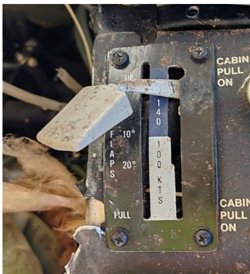
Figures 9 and 10: Flap and cowl flap selectors. (Source: Investigator)
