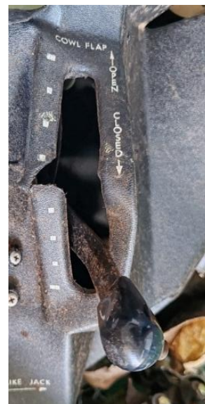
Figures 9 and 10: Flap and cowl flap selectors. (Source: Investigator)
