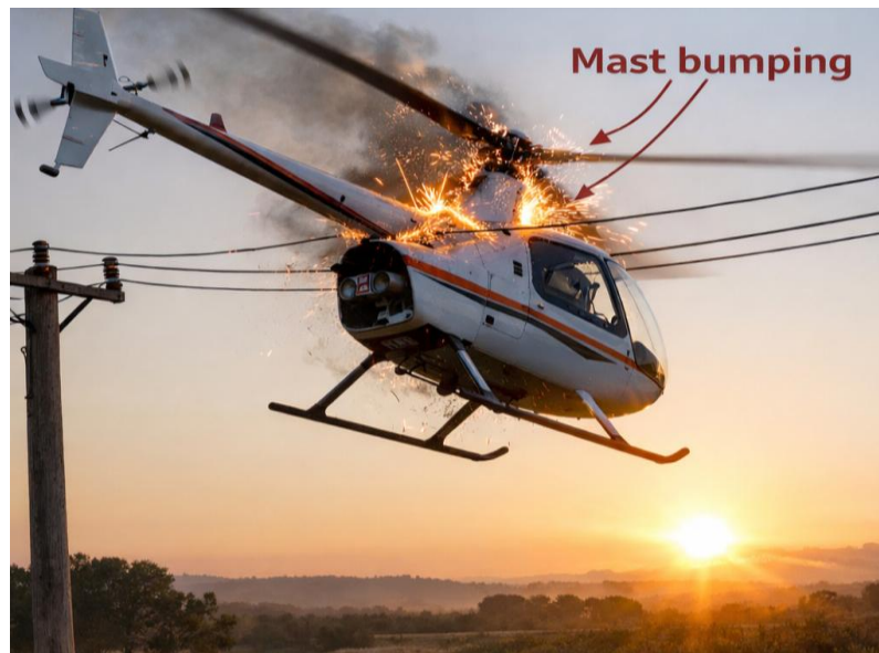
Figure 7: Illustration of mast bumping (this is not the aircraft that was involved in the accident).
